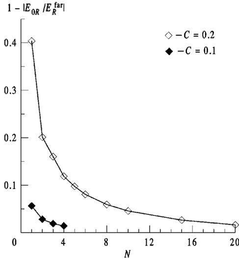
FIG. 2. The difference between the reflected wave field in the far zone, calculated under ( $E_R^{far}$ ) and without ( $E_{0R}$ ) the consideration of the discrete structure of the medium, as a function of the number of monolayers  $N$  which constitute the film. The calculations are performed for the cubic lattice. The parameters are  $k_0 = 0.01 \text{ nm}^{-1}$ ;  $a = 0.5 \text{ nm}$ ;  $\Theta_I = 0^\circ$ .
