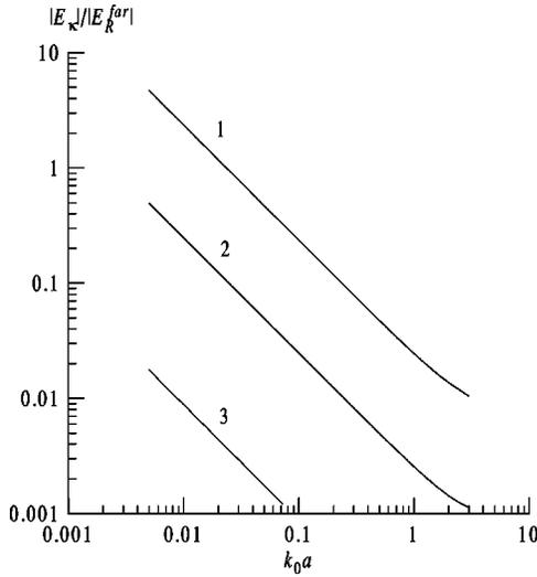
FIG. 4. The ratio of the evanescent field amplitudes near the surface  $E_\kappa$  to the amplitude of the reflected field in the wave zone  $E_R^{far}$ . The calculations are performed for the cubic lattice. The parameters are  $k_0=0.01 \text{ nm}^{-1}$ ;  $\Theta_I=0$ ; the distance between the observation point and the surface is equal to  $a$ ; 1 –  $|E_1/E_R^{far}|$ ; 2 –  $|E_2/E_R^{far}|$ ; 3 –  $|E_4/E_R^{far}|$ .
