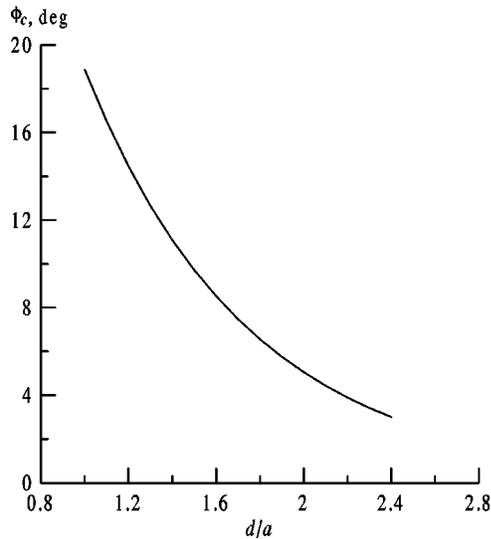
FIG. 9. The angle between the minimal contrast direction and the polarization vector of the external wave  $\phi_c$  as a function of the distance to the film surface  $d$ . The calculations are performed for the cubic lattice,  $\Theta_I = 0^\circ$ .
