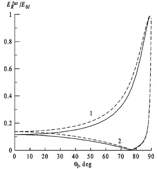
FIG. 3. The dependence of the electric-field strength amplitude of the reflected wave  $E_R^{far}$  on the incident angle of the external wave  $\Theta_I$  in the wave zone for  $s$  (1) and  $p$  (2) polarizations: — under consideration of the discrete structure; --- according to the Airy formulas. The calculations are performed for the cubic lattice. The parameters are  $k_0 = 0.01 \text{ nm}^{-1}$ ;  $a = 0.5 \text{ nm}$ ;  $N = 3$ ;  $C = 0.2$ .
