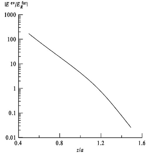
FIG. 5. Coordinate dependences of the ratio of the total amplitude of the evanescent waves  $E^{ev}$  to the amplitude of the reflected wave field in the wave zone  $E_R^{far}$ . The calculations are performed for the cubic lattice. The parameters are:  $k_0=0.01 \text{ nm}^{-1}$ ;  $a=0.5 \text{ nm}$ ;  $\Theta_I=0^\circ$ . The observation point is above an atom of the film.
