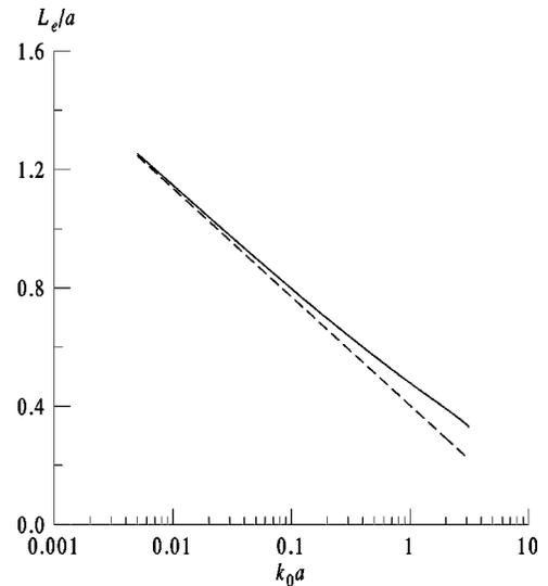
FIG. 6. The dependence of the distance  $L_e$ , at which the amplitudes of the evanescent and propagating parts of the reflected wave field are equal to one another, on the parameter  $k_0 a$ : — exact numerical calculations; --- an estimate according to formula (42). The calculations are performed for the cubic lattice,  $\Theta_I=0^\circ$ .
