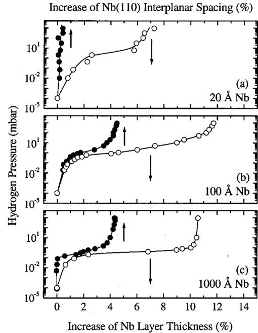
FIG. 3. Comparison between hydrogen-induced relative increase of the out-of-plane Nb(110) interplanar spacing (filled symbols), and increase of Nb layer thickness (open symbols) in Fe/Nb multilayers for various hydrogen pressures.
