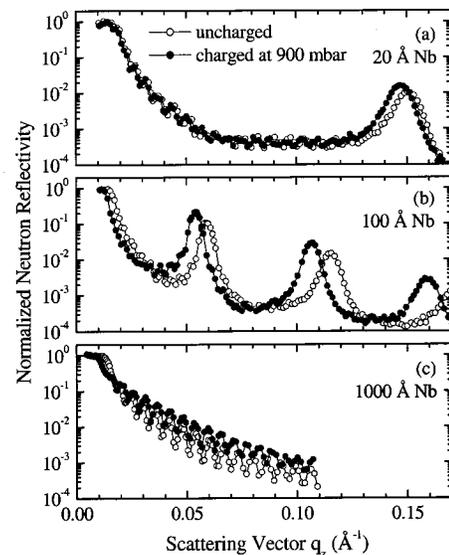
FIG. 1. Neutron reflectivity curves of Fe/Nb multilayers with various Nb layer thicknesses, measured after sample preparation (open symbols) and at a hydrogen pressure of 900 mbar (filled symbols).
