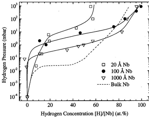
FIG. 2. Hydrogen solubility curves of Fe/Nb multilayers with various Nb layer thicknesses at  $T=185$  °C. The dashed line for bulk Nb is extrapolated from literature.
