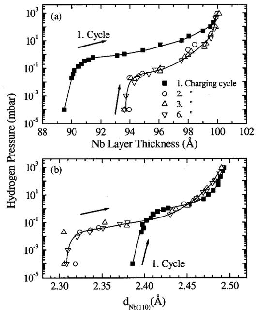
FIG. 5. (a) Expansion of Nb layer thickness upon repeated hydrogen charging and decharging, and (b) corresponding expansion of Nb(110) lattice planes in Fe/Nb multilayers.
