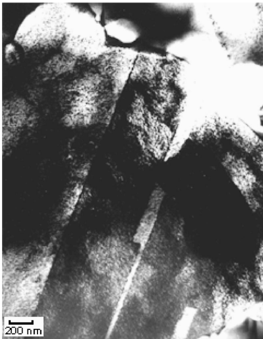
FIG. 10. The bright field TEM image of UFG Cu annealed up to 400 °C. The specimen exhibits a fully recrystallized microstructure. The small black dots are only artifacts of ion milling of the specimen prior to measurement.
