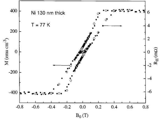
FIG. 1. Hall resistance (solid circles, right-hand axis) and magnetization (open circles, left-hand axis) of 130-nm-thick Ni film measured at 77 K with magnetic field  $B_0$  perpendicular to the film plane.
