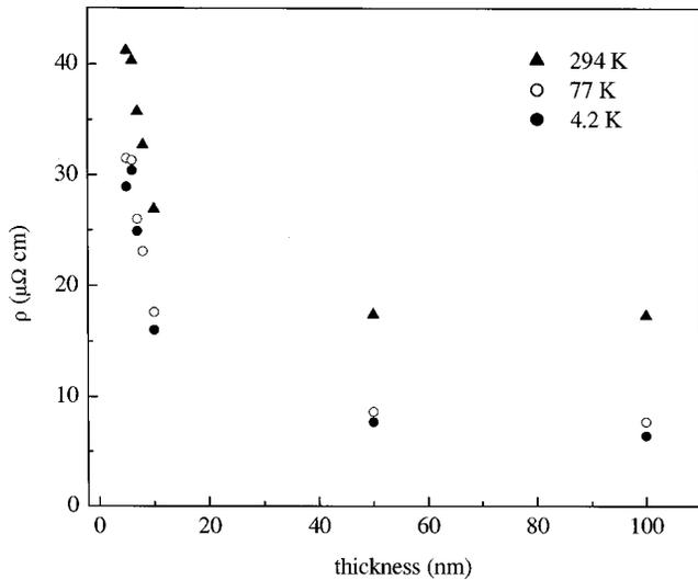
FIG. 2. Resistivity of Ni films as a function of their thickness at 294, 77, and 4.2 K.
