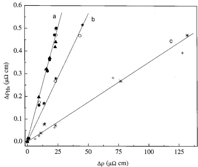
FIG. 10. Surface scattering component of the extraordinary Hall resistivity as a function of the respective resistivity term for (a) high-quality thin Ni films, (b) “low”-quality Ni films, and (c) Ni-SiO<sub>2</sub> mixtures. Group (a) is shown for three temperatures: 294, 77, and 4.2 K. Groups (b) and (c) are shown for 294 and 77 K. Straight lines are guides for the eyes.
