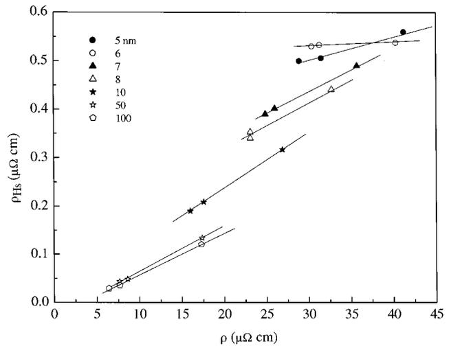
FIG. 4. Extraordinary Hall resistivity of Ni samples as a function of their total resistivity. Three data points per sample correspond to three temperatures 294, 77, and 4.2 K. Straight lines are guides for the eyes.
