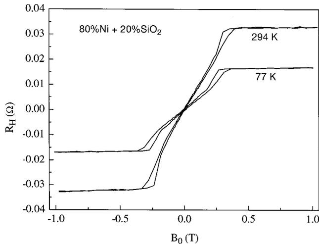
FIG. 9. Hall resistance of the Ni-SiO<sub>2</sub> granular film as a function of applied magnetic field. Ni volume concentration is 80%. Thickness is about 200 nm.
