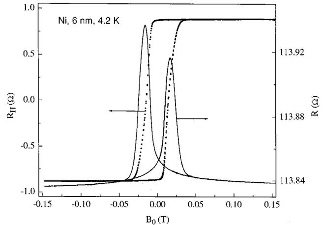
FIG. 8. Hall resistance (solid circles, left-hand axis) and longitudinal resistance (solid line, right-hand axis) as a function of applied magnetic field of (a) 8-nm- and (b) 6-nm-thick Ni films.  $T = 4.2$  K.
