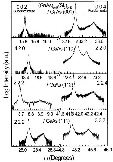
FIG. 2. Fundamental and superstructure reflections rocking curves of  $(\text{GaAs})_{0.57}(\text{Si}_2)_{0.43}$  epitaxially grown on (a) (001), (b) (110), (c) (112), and (d) (111) GaAs.
