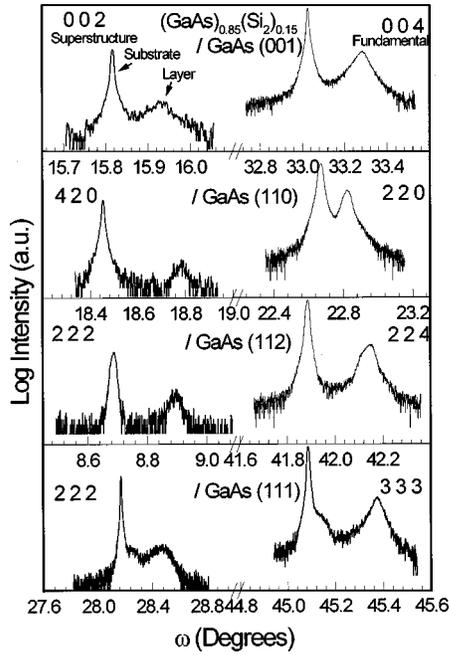
FIG. 1. Typical diffraction profiles of fundamental and superstructure reflections obtained by HRXRD for  $(\text{GaAs})_{0.85}(\text{Si}_2)_{0.15}$  metastable alloys epitaxially grown on (a) (001), (b) (110), (c) (112), and (d) (111) GaAs.
