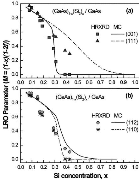
FIG. 3. Experimental and modeled long-range order parameter behavior with Si concentration of  $(\text{GaAs})_{1-x}(\text{Si}_2)_x$  epitaxially grown on (a) (001) and (111) and (b) (110) and (112) GaAs.
