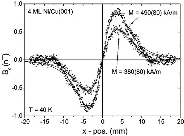
FIG. 1. Measured (data points) and calculated (lines) stray-field distributions for 4 ML Ni/Cu(001) at 40 K before (larger signal) and after Cu capping (smaller signal). A clear reduction of the stray field due to Cu capping is revealed. The fitted magnetizations are given as well.
