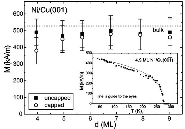
FIG. 2. Measured remanent magnetizations at 40 K for a series of Ni/Cu(001) films between 4 and 9 ML before (solid squares) and after (open circles) Cu capping. All films present bulklike magnetizations except the Cu-capped 4 ML one which shows a decreased magnetization by about 22%. From the temperature dependence of the magnetization shown in the inset one can extract the magnetic moments given in Table I.
