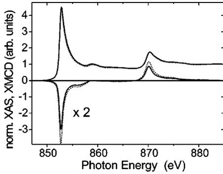
FIG. 3. Normalized x-ray absorption spectra (XAS, linear light) and XMCD (circular light) spectra for Cu/20 ML Ni/Cu(001) (dashed) and Cu/4 ML Ni/Cu(001) (solid line). A clear reduction of the XMCD signal and, consequently, reduction of the magnetic moment is observed by decreasing the Ni thickness yielding  $0.44(5)\mu_B/\text{atom}$ . The measurement was carried out at 10 K under a field of 3 T applied along the film normal (hard axis).
