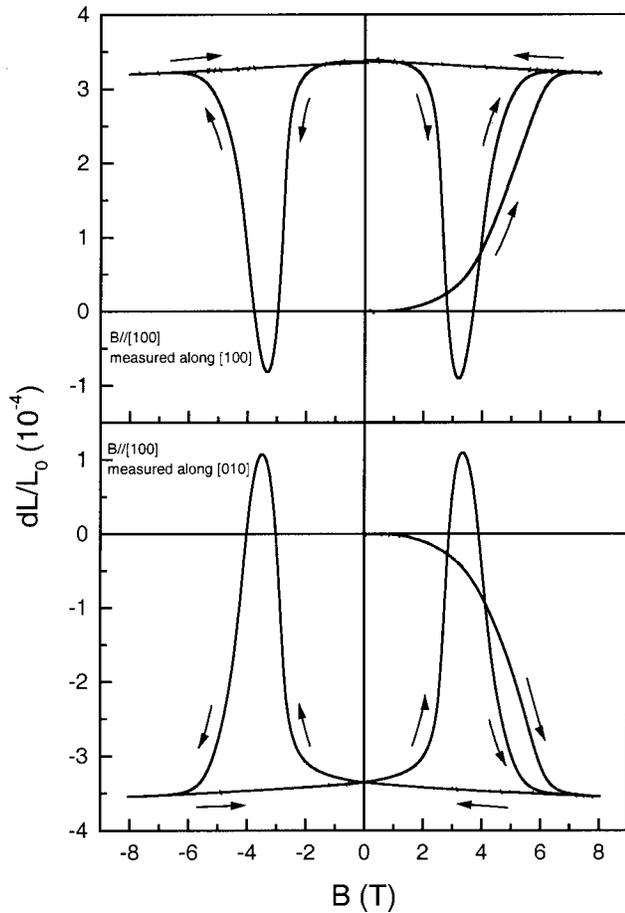
FIG. 3. Field dependence of the magnetostriction at 5 K measured (a) in the [100] direction and (b) in the [010] direction on a single crystal of the approximate formula composition  $\text{TbFe}_{4.4}\text{Al}_{7.6}$  with the field applied along the [100] direction.
