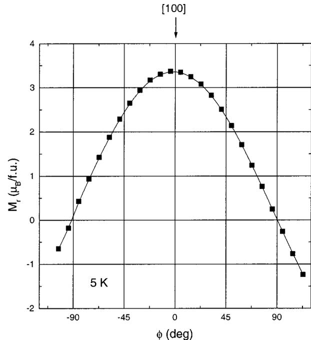
FIG. 2. Dependence of the remanence at 5 K measured in zero field in various directions in the basal plane on a single crystal of the approximate formula composition  $\text{TbFe}_{4.4}\text{Al}_{7.6}$  after the crystal had been magnetized in a field of 9 T in the  $[100]$  direction and the field has subsequently been reduced to zero.
