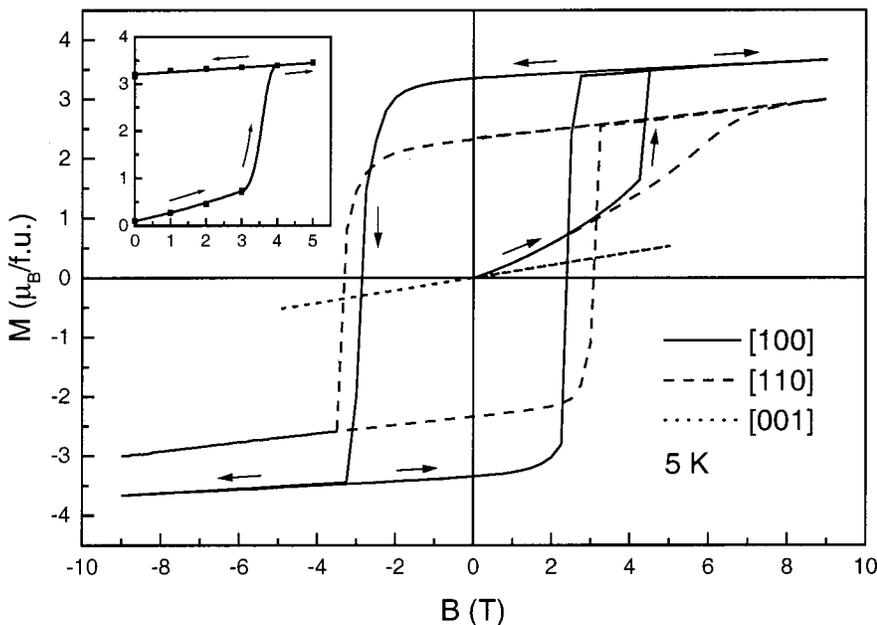
FIG. 1. Field dependence of the magnetization at 5 K measured on a single crystal of the approximate formula composition  $\text{TbFe}_{4.4}\text{Al}_{7.6}$  with the field applied in the [100], [110], and [001] direction. The inset shows the field dependence in the [010] direction after the crystal had been magnetized in a field of 9 T in the [100] direction and the field has subsequently been reduced to zero.
