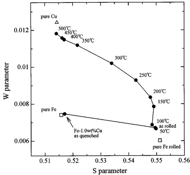
FIG. 2. Result of  $S$ - and  $W$ -parameter correlations ( $S$ - $W$  plot) for an Fe-1.0 wt % Cu alloy quenched and 20% rolled, followed by a subsequent isochronal annealing up to 500 °C together with those for pure bulk Cu and Fe, a pure 20% rolled Fe alloy, and a Fe-1.0 wt % as-quenched Cu alloy.
