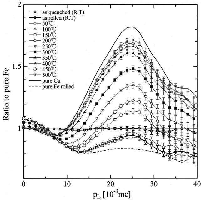
FIG. 1. CDB ratio curves [momentum distribution normalized to that of annealed (defect-free) pure Fe] of an Fe-1.0 wt % Cu alloy, quenched and then 20% rolled, followed by a subsequent isochronal annealing up to 500 °C, together with the curves for pure bulk Cu, a pure Fe 20% rolled alloy, and an Fe-1.0 wt % Cu as-quenched alloy.
