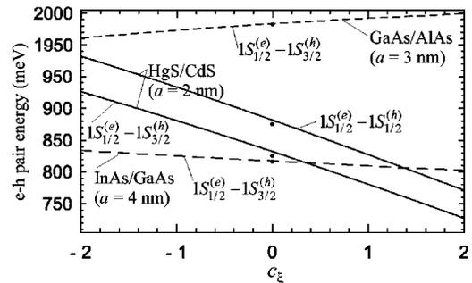
FIG. 10. The lowest electron-hole pair energies in different QDH's as a function of  $c_{\xi}$  ( $\chi \neq 0$ ). Each dot is related to the closest curve and indicates the corresponding result of the symmetrized model ( $c_{\xi}=0, \chi=0$ ).
