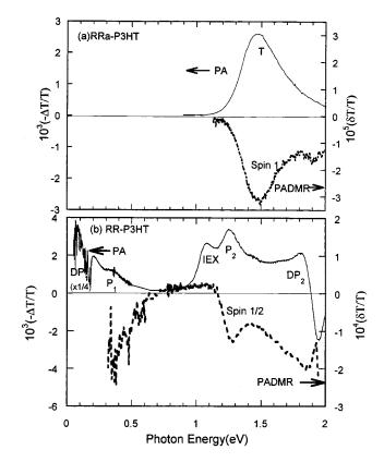
FIG. 5. Cw PA and  $\lambda$ -PADMR spectra of RR*a*-P3HT (a) and RR-P3HT (b) films measured at 10 K. The  $\lambda$ -PADMR in (a) was measured at  $H_{1/2}$ = 430 G, which corresponds to transitions among spin-1 triplet sublevels at  $g \approx 5.1$ , whereas in (b) it was measured at H = 1006 G, which corresponds to transitions among spin- $\frac{1}{2}$  doublet sublevels at  $g \approx 2$ . Several PA bands are assigned.
