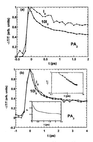
FIG. 4. Transient decays of PA<sub>2</sub> (a) and PA<sub>3</sub> (b) bands in RR-P3HT at two different excitation intensities of  $I_0$  of 20  $\mu$ J/cm<sup>2</sup> and 10 $I_0$  (or 200  $\mu$ J/cm<sup>2</sup>), respectively. The upper inset in (b) shows the PA<sub>3</sub> decay in logarithmic scale and a power-law fit to the data, whereas the lower inset shows its polarization memory decay P(t).
