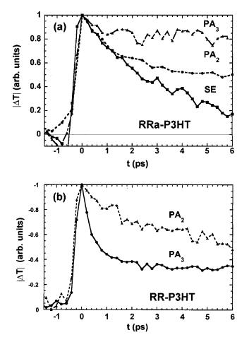
FIG. 3. Transient PA and SE decays in RRa-P3HT (a) and RR-P3HT (b), up to 6 ps.
