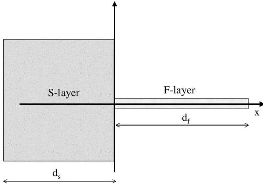
FIG. 1. Geometry of the  $S/F$  system.
