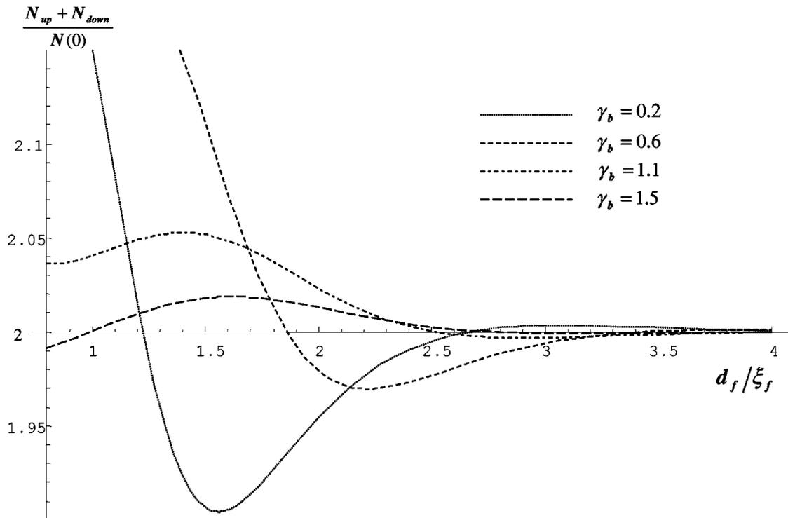
FIG. 5. Variation of the normalized local density of states ( $N_{tot}$ ) at zero energy as a function of the  $F$  layer thickness normalized by the coherence length  $\xi_f$ . The different curves are obtained for different values of the transparency coefficient  $\gamma_b$  ( $\gamma_b=0.2$ ,  $\gamma_b=0.6$ ,  $\gamma_b=1.1$ ,  $\gamma_b=1.5$ ).
