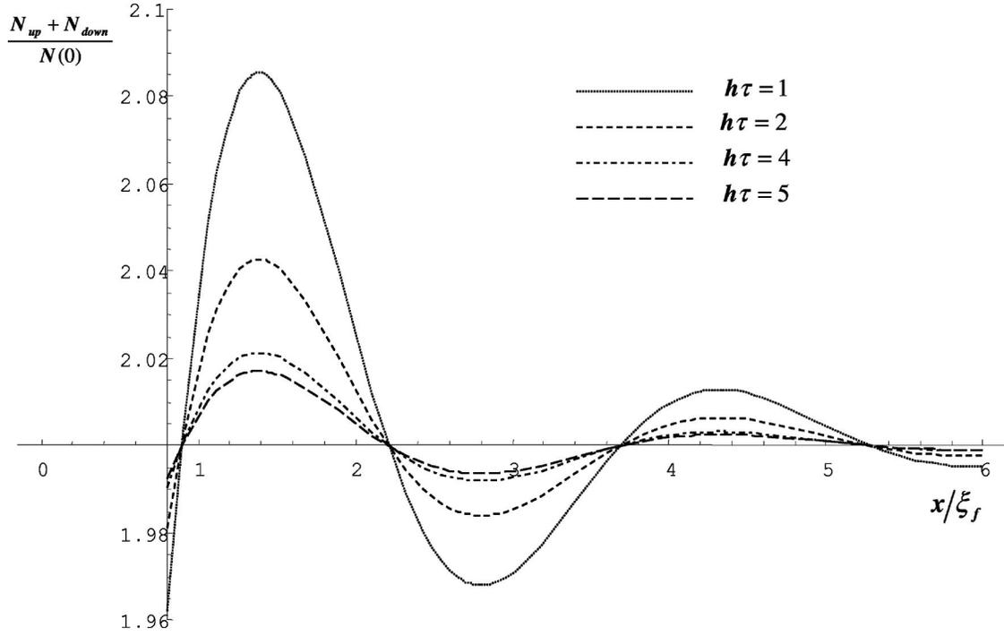
FIG. 2. Variation of the normalized density of states at low energy ( $\omega=0.1h$ ) in the ferromagnet as a function of the normalized distance  $x/\xi_f$  to the  $S/F$  interface. The different curves correspond to different values of the parameter  $h\tau$  ( $h\tau=1, h\tau=2, h\tau=3, h\tau=4, h\tau=5$ ). The parameter  $\bar{\Delta}=\Delta/h$  is chosen to be 0.05.
