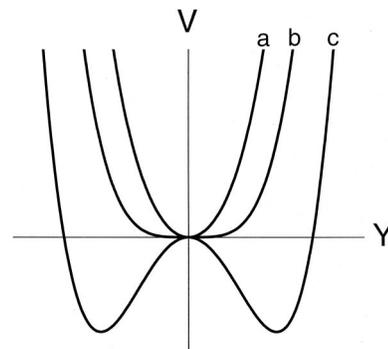
FIG. 1. Potential energy  $V$  as a function of the fundamental mode displacement  $Y$ . This function is harmonic above critical strain  $\varepsilon > \varepsilon_c$  (a), quartic at critical strain  $\varepsilon = \varepsilon_c$  (b), and a double-well below,  $\varepsilon < \varepsilon_c < 0$  (c).
