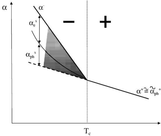
FIG. 1. Sketch of the behavior of the thermal diffusivity for a high- $T_c$  superconductor (continuous line) as a function of temperature. The broken line ( $\tilde{\alpha}^+$ ) is the extrapolated normal thermal diffusivity below  $T_c$ ; the shadowed area represents the superconducting phase contribution made of  $\alpha_e^s$  and  $\alpha_{ph}^s$  below  $T_c$ . The line separating  $\alpha_e^s$  and  $\alpha_{ph}^s$  is merely indicative.
