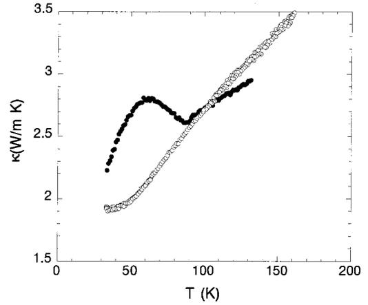
FIG. 3. Comparison of the thermal conductivity of  $\text{DyBa}_2\text{Cu}_3\text{O}_7$  (●) and  $\text{DyBa}_2\text{Cu}_3\text{O}_{6.3}$  (○) versus temperature.
