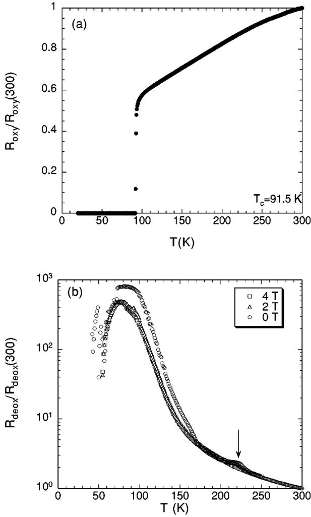
FIG. 2. (a) Normalized resistance of a  $\text{DyBa}_2\text{Cu}_3\text{O}_7$  sample versus temperature. (b) Normalized resistance of the sample when it is deoxygenized to be  $\text{DyBa}_2\text{Cu}_3\text{O}_{6.3}$ . The data is shown when different magnetic fields are applied versus temperature in a semi log plot. The arrow indicates the antiferromagnetic transition.
