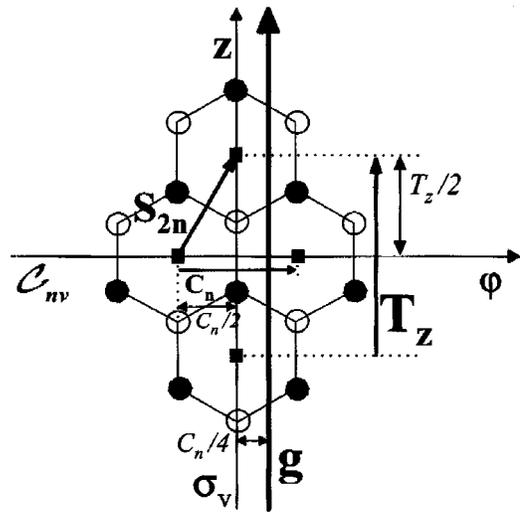
FIG. 3. 2D projection of various symmetries in zigzag BN-NT's ( $\bullet$ , B;  $\circ$ , N):  $T_z$  is the primitive translation;  $S_{2n}$  is the screw axis with nonprimitive translation and rotation, denoted by  $T_z/2$  and  $C_n/2$ , respectively;  $g$  is a glide plane;  $C_{nv}$  stands for the corresponding point-group operations, among which  $\sigma_v$  and  $C_n$  are denoted.
