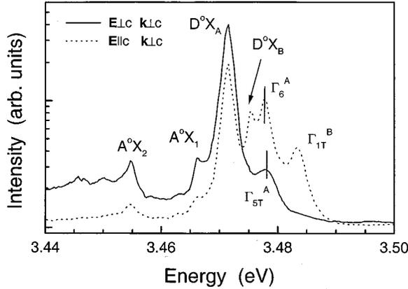
FIG. 3. Polarized spectra of a free-standing GaN sample for  $\mathbf{E}\perp c, \mathbf{k}\perp c$  (solid line), and  $\mathbf{E}\parallel c, \mathbf{k}\perp c$  (dotted line).
