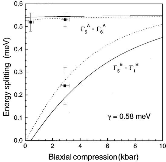
FIG. 5. Stress dependence of the energy splitting  $\Gamma_5^A - \Gamma_6^A$  and  $\Gamma_5^B - \Gamma_1^B$  calculated with parameters  $\Delta_1 = 10$  meV,  $\Delta_2 = 6.2$  meV,  $\Delta_3 = 5.5$  meV, and  $C_3 = 4.91$  eV (Ref. 29) (solid lines) and  $\Delta_1 = 10$  meV,  $\Delta_2 = 5.5$  meV,  $\Delta_3 = 6.0$  meV, and  $C_3 = 7.2$  eV (Ref. 30) (dotted lines). The squares represent the experimentally obtained values.
