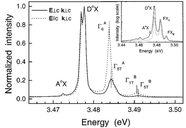
FIG. 2. Normalized photoluminescence spectra of a 80- $\mu\text{m}$ -thick GaN layer for  $\sigma$  polarization (solid line) and  $\pi$  polarization (dotted line). The inset shows the spectra in a logarithmic scale.
