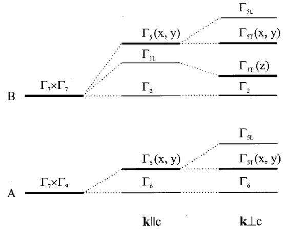
FIG. 4. Schematic diagram of the internal structure of  $A$  and  $B$  excitons in a wurtzite GaN. The allowed polarizations are given in parentheses. Thin lines correspond to dipole-forbidden states.
