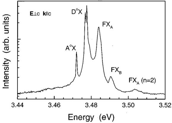
FIG. 1. Unpolarized photoluminescence spectrum of a 80- $\mu\text{m}$ -thick GaN layer for the  $\mathbf{k}\parallel c$  configuration.
