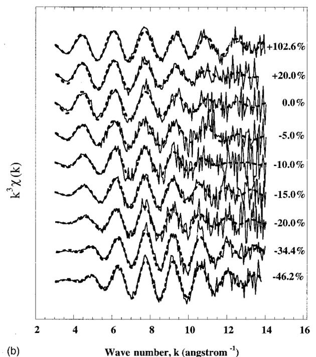
FIG. 2.  $k^3$ -weighted Ge  $K$ -edge EXAFS spectra of  $\text{Ge}_x\text{As}_y\text{S}_{1-x-y}$  glasses with (a)  $x:y=1:1$  and (b)  $x:y=2.5:1$ . The %S in excess of stoichiometry for each glass composition is indicated alongside each spectrum. Solid lines represent experimental data and dashed lines correspond to least-squares fits obtained using EXCURV92.
