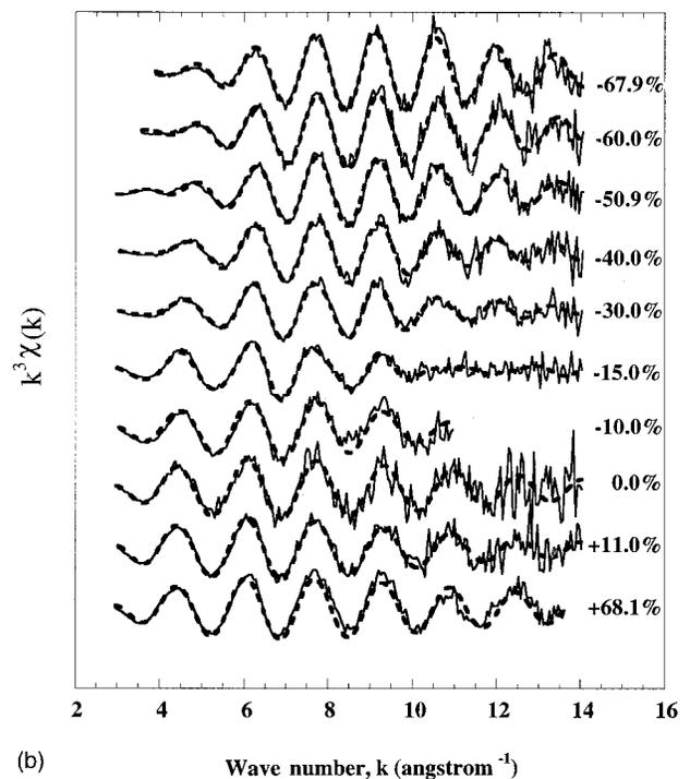
FIG. 8.  $k^3$ -weighted (a) Ge and (b) As  $K$ -edge EXAFS spectra of  $Ge_xAs_yS_{1-x-y}$  glasses with  $x:y = 1:2$ . The %S in excess of stoichiometry for each glass composition is indicated alongside each spectrum. Solid lines represent experimental data and dashed lines correspond to least-squares fits obtained using EXCURV92.
