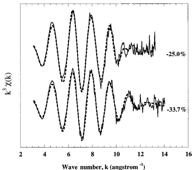
FIG. 11.  $k^3$ -weighted Ge  $K$ -edge EXAFS spectra of binary  $\text{Ge}_x\text{S}_{1-x}$  glasses. The %S in excess of stoichiometry for each glass composition is indicated alongside each spectrum. Solid lines represent experimental data and dashed lines correspond to least-squares fits obtained using EXCURV92.
