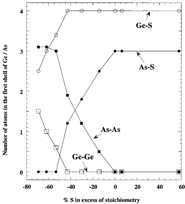
FIG. 6. Compositional variation in the atomic make-up of the first coordination shell of Ge and As atoms in  $Ge_xAs_yS_{1-x-y}$  glasses with  $x:y = 1:1$ , as derived from fitting the Ge and As  $K$ -edge EXAFS data. Solid lines through the data points are guides to the eye only.
