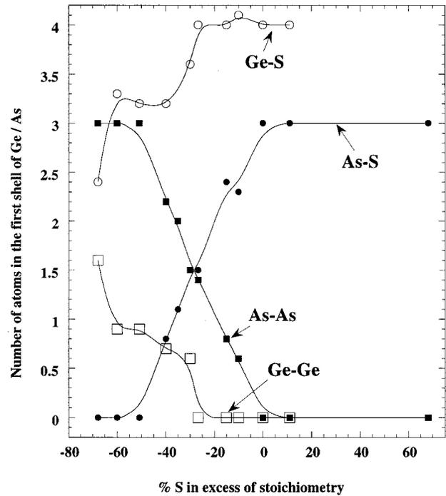
FIG. 10. Compositional variation in the atomic make-up of the first coordination shell of Ge and As atoms in  $\text{Ge}_x\text{As}_y\text{S}_{1-x-y}$  glasses with  $x:y=1:2$ , as derived from fitting the Ge and As  $K$ -edge EXAFS data. Solid lines through the data points are guides to the eye only.
