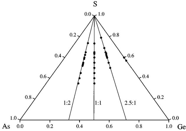
FIG. 1. Ternary plot of the  $\text{Ge}_x\text{As}_y\text{S}_{1-x-y}$  glass compositions investigated in this study.
