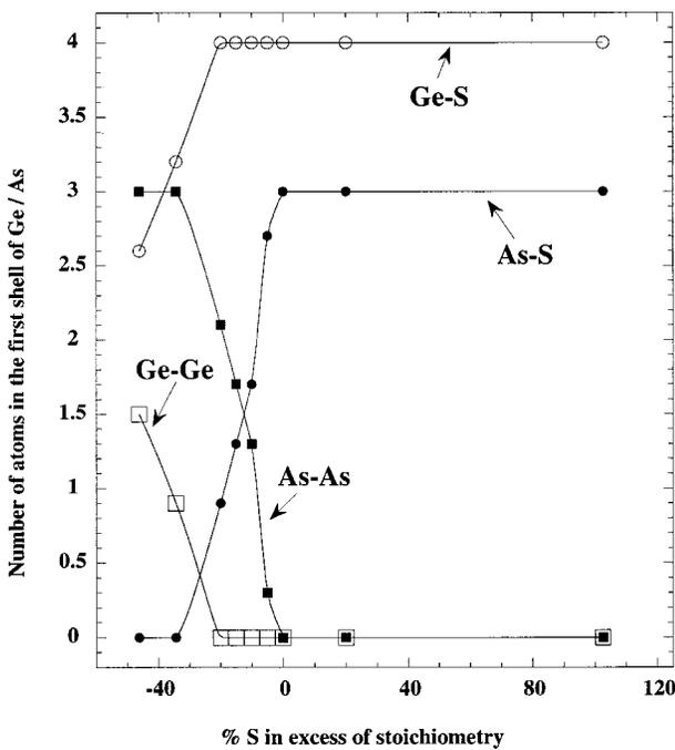
FIG. 7. Compositional variation in the atomic make-up of the first coordination shell of Ge and As atoms in  $Ge_xAs_yS_{1-x-y}$  glasses with  $x:y = 2.5:1$ , as derived from fitting the Ge and As  $K$ -edge EXAFS data. Solid lines through the data points are guides to the eye only.
