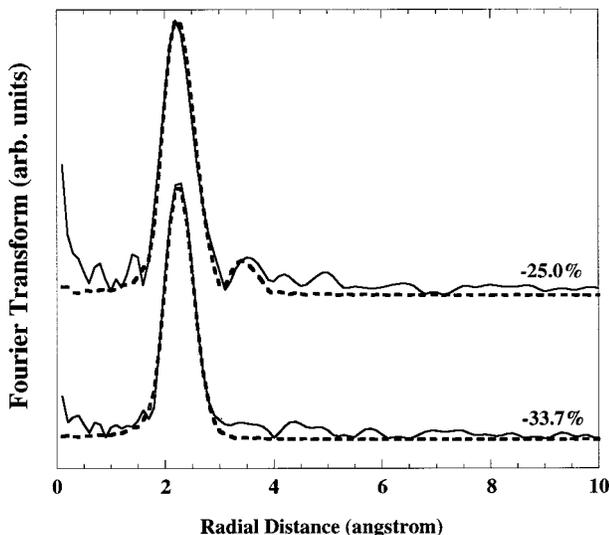
FIG. 12. Magnitudes of the Fourier-transform of the  $k^3$ -weighted Ge  $K$ -edge EXAFS spectra of  $\text{Ge}_x\text{S}_{1-x}$  glasses with various levels of S in excess of stoichiometry. Solid lines represent experimental data and dashed lines correspond to least-squares fits obtained using EXCURV92.
