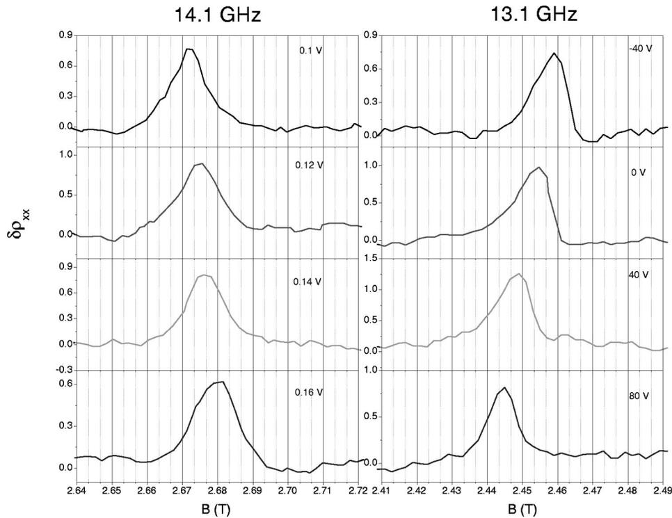
FIG. 3. Electrically detected electron spin resonance spectra at a sequence of gate voltages for (a) a front gate and (b) a back gate. For the front gate case, the resonant peak moves progressively to higher magnetic field when the amplitude of the bias gate voltage is increased. In contrast, the peak shifts towards lower field for the back gate case. (The smooth non-resonant background of the signal was subtracted for clarity.)
