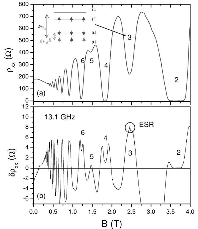
FIG. 2. (a) Typical trace of the resistivity  $\rho_{xx}$  as a function of the magnetic field. Landau level filling factors  $\nu$  are indicated. Inset: energy diagram for the case of  $\nu=3$ . (b) The microwave radiation induced resistivity change  $\delta\rho_{xx}$ . Note the ESR feature around  $\nu=3$ .
