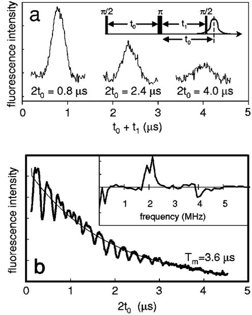
FIG. 2. Optically detected spin echoes and the envelope of the spin echo decay. In (a), the inset illustrates the pulse sequence used. (b) shows the spin echo decay envelope with nuclear modulation; the overall decay of the envelope is  $3.6 \mu\text{s}$ . The inset shows the cosine Fourier transform of the modulation.
