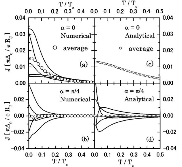
FIG. 4. The Josephson current in dirty SNS junctions is shown as a function of the temperatures. The numerical results for  $\alpha_{L,R} = 0$  and  $\pi/4$  are plotted in (a) and (b), respectively. The lines are the numerical results of several samples with different random configurations and the open circles are the average over a number of samples. For comparison, we show the analytical results for  $\alpha_{L,R} = 0$  in (c) and for  $\pi/4$  in (d).
