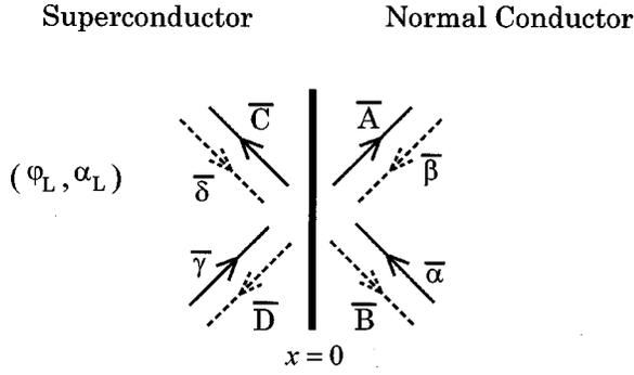
FIG. 5. The transmission and the reflection coefficients at the left NS interface. There are four incoming and outgoing channels.
