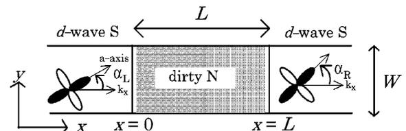
FIG. 1. The SNS junction of the  $d$ -wave superconductor is illustrated. The orientation angle in the left (right) superconductor is  $\alpha_L$  ( $\alpha_R$ ).
