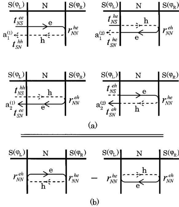
FIG. 2. The reflection coefficients in (a) contribute to the Josephson current proportional to  $\sin(\varphi_L - \varphi_R)$ . The Josephson current calculated from the four reflection coefficients in (a) is summarized in a reflection process in (b).
