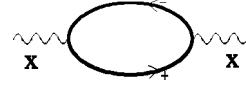
FIG. 4. Bubble diagram contributing to the diagonal conductivity \tilde{\sigma}_{xx} . The signs +/- refer to the retarded/advanced average Green's function \underline{G}^\pm .
