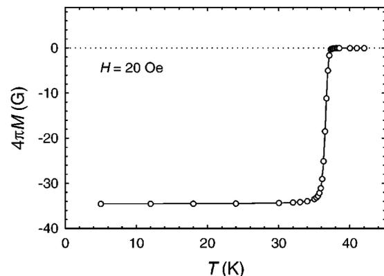
FIG. 1. Zero-field-cooled magnetization,  $M(T)$ , of MgB<sub>2</sub> for  $H = 20$  Oe. This curve reveals the superconducting transition temperature  $T_c$  and the transition width  $\Delta T_c$  to be about 37 K and 1 K, respectively.
