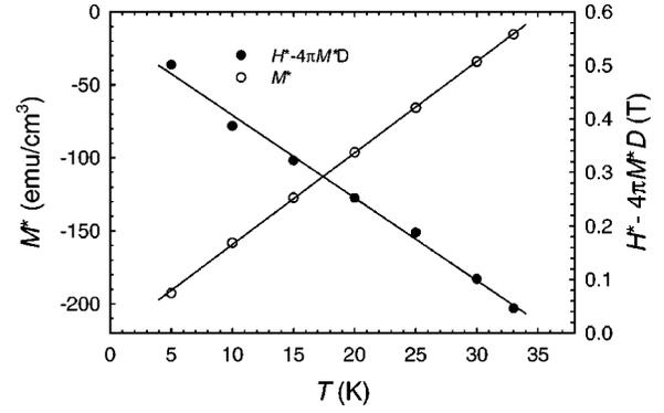
FIG. 4. Temperature dependence of phenomenological parameters  $M^*$  and  $H^* - 4\pi M^*D$ , where  $D$  is the demagnetization factor of the sample. Solid lines represent linear least-squares fits of the data.
