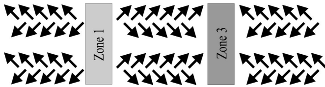
FIG. 8. Schematic representation of the orientation of the electronic lone pair in the [BiO] layers.
