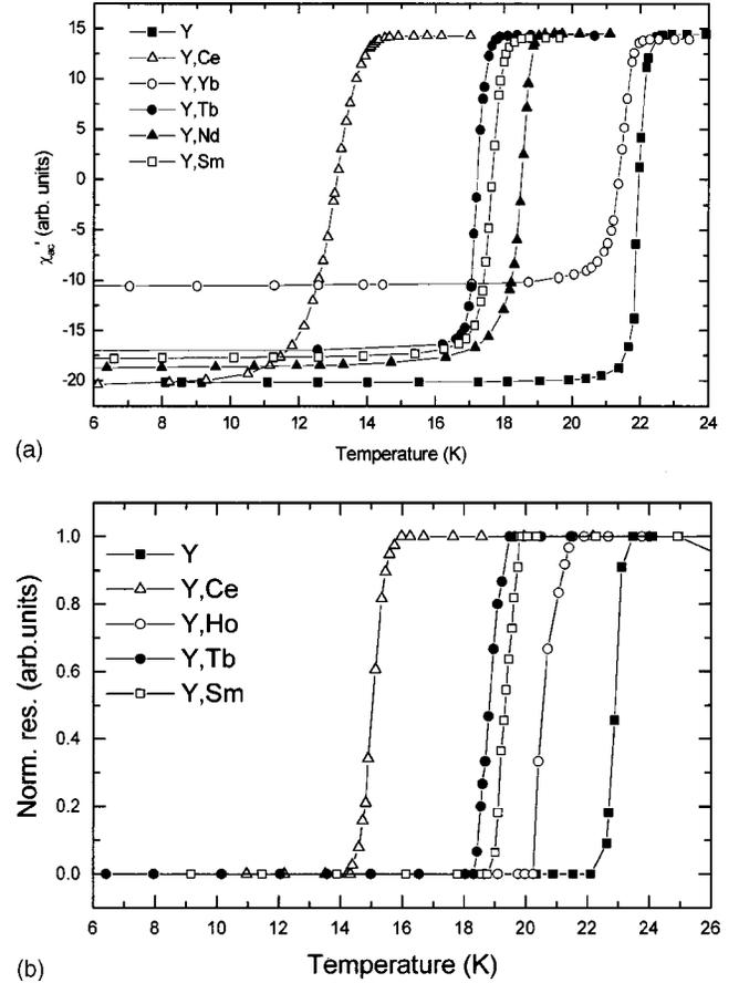
FIG. 2. (a) ac susceptibility  $\chi_{ac}$  and (b) dc resistivity for  $Y_{0.9}R_{0.1}Pd_5B_3C_{0.35}$  as a function of temperature; different symbols correspond to different  $R$  ions as indicated in figures. The lines are guides for the eye.
