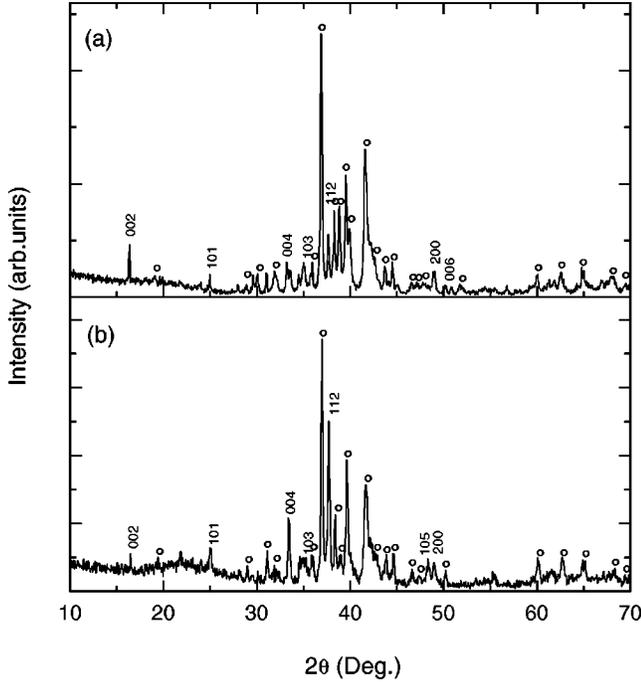
FIG. 1. X-ray-diffraction patterns of  $RPd_5B_3C_{0.35}$ ; (a)  $R=Y$  and (b)  $R=Dy$ . The indexed lines correspond to the tetragonal phase  $RPd_2B_2C$  and open-circle-marked lines correspond to the orthorhombic  $RPd_7B_4$  phase.
