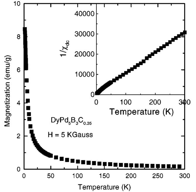
FIG. 4. dc magnetization versus temperature for  $DyPd_5B_3C_{0.35}$ . The inset shows the inverse of dc susceptibility ( $1/\chi_{dc}$ ) versus temperature for the two materials.
