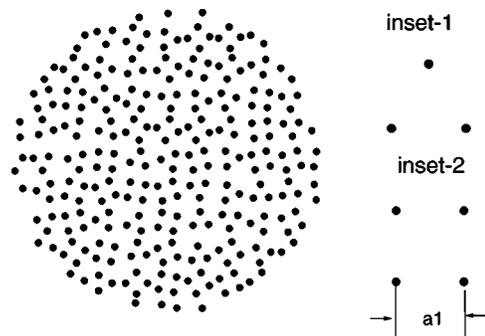
FIG. 6. Schematic of another amorphous photonic structure. Here we apply two unit cells, square and triangle, to form this kind of APM. Both of these two units have the same sidelength  $a_1 = 10$  mm, as shown in insets 1 and 2. Then a square lattice with lattice constant  $a_2 = 10$  mm is produced. Finally each lattice point is randomly replaced by any one of the basic units, and these units are rotated randomly around their own centers, respectively.
