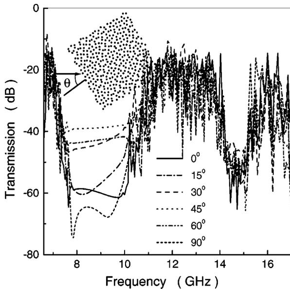
FIG. 4. The transmission spectra of the amorphous photonic material with various incident angles. The photonic structure is shown in the inset. The size of the APM is  $200 \times 200$  mm, where,  $a_1 = 10$  mm,  $a_2 = 20$  mm,  $r = 2.5$  mm,  $\epsilon_a = 12.0$ , and  $\epsilon_b = 1.0$ . The calculations are carried out at six angles between  $0^\circ \sim 90^\circ$ . It can be seen that the gap position is independent of incident angles.
