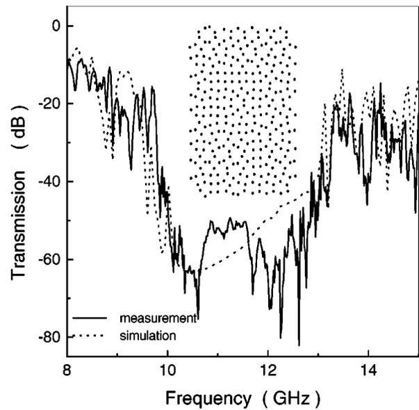
FIG. 5. The comparison between measured and calculated transmission spectra for the amorphous photonic material fabricated by the first method and shown in the inset, where  $a_1 = 10$  mm,  $a_2 = 20$  mm,  $\epsilon_a = 8.4$ , and  $\epsilon_b = 1.04$ .
