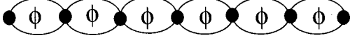
FIG. 1. A quasi-one-dimensional chain with sites connected to each other by two hopping paths. Each loop is threaded by a uniform magnetic flux \phi .
