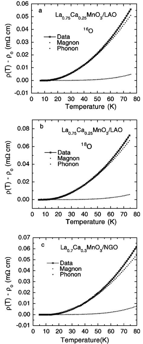
FIG. 4. The temperature-dependent part of the resistivity at low temperatures (below  $T_C/3$ ) for the  $\text{La}_{1-x}\text{Ca}_x\text{MnO}_3$  films. The solid lines are fitted curves by Eq. (3) with a fixed  $\alpha=4.5$ . Plotted is also the respective contribution from the two-magnon scattering (solid circle) or from the soft optical phonon scattering (solid triangle).
