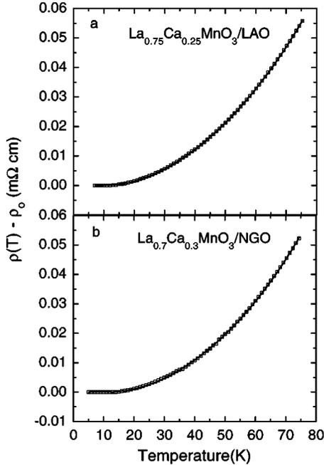
FIG. 3. The temperature-dependent part of the resistivity at low temperatures for the  $\text{La}_{1-x}\text{Ca}_x\text{MnO}_3^{16}\text{O}$  films with  $x=0.25$  and  $0.30$ . The solid lines are fitted curves by Eq. (3) with a fixed  $\alpha=5$ .
