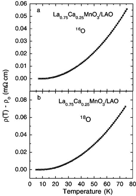
FIG. 2. The temperature-dependent part of the resistivity at low temperatures (below  $T_C/3$ ) for the  $^{16}\text{O}$  and  $^{18}\text{O}$  films of  $\text{La}_{0.75}\text{Ca}_{0.25}\text{MnO}_3$ . The solid lines are the fitted curves by Eq. (3) using four fitting parameters  $\alpha$ ,  $A$ ,  $B$ , and  $\omega_s$ . The best fits lead to  $\alpha=4.0\pm 0.3$  for the  $^{16}\text{O}$  sample and  $\alpha=4.0\pm 0.4$  for the  $^{18}\text{O}$  sample.
