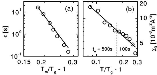
FIG. 3. Double-logarithmic plots of (a)  $\tau = (2\pi f)^{-1}$  vs  $T_m/T_g - 1$  and (b)  $\chi_3$  vs  $T/T_g - 1$  (obtained after waiting times  $t_w$  as indicated) for the DMIM with  $t = 1.0$  nm, where  $T_g = (47.1 \pm 5.3)$  and  $(50.7 \pm 2.3)$  K, respectively, from best fits to power laws (straight lines).
