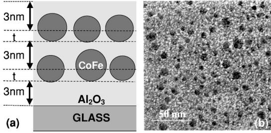
FIG. 1. (a) Schematic cross section of a DMIM consisting of substrate,  $\text{Al}_2\text{O}_3$  layers (thickness 3 nm) and CoFe layers ( $t$ ) forming quasispherical nanoparticles, and (b) transmission top view electron micrograph of a CoFe ( $t = 1.3$  nm)/ $\text{Al}_2\text{O}_3$  ( $t = 3$  nm) bilayer, (Ref. 15) where dark circles indicate CoFe nanoparticles embedded into gray-scaled  $\text{Al}_2\text{O}_3$ .
