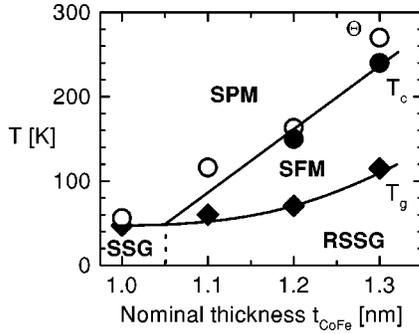
FIG. 5. Magnetic phase diagram of CoFe/Al<sub>2</sub>O<sub>3</sub> DMIM's vs nominal CoFe thickness  $t$  showing interpolating phase lines SPM-SFM ( $T_c$  vs  $t$ ) and SFM-RSSG ( $T_g$  vs  $t$ ) together with Curie temperatures,  $\Theta$  vs  $t$ , and the tentative vertical SSG-RSSG line (SPM=superparamagnetic, SFM=superferromagnetic, RSSG=reentrant superspin glass, and SSG=superspin glass).
