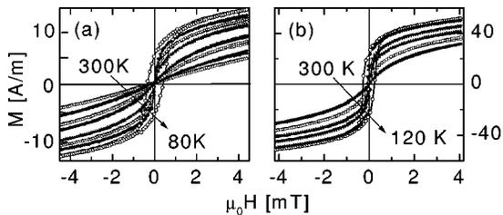
FIG. 4. Low-field magnetization curves  $M$  vs  $\mu_0 H$  obtained on the DMIM with  $t = 1.2$  (a) and  $1.3$  nm (b) after ZFC from  $300$  K to (a)  $300, 260, 220, 180, 140, 120, 100, 80$  K and (b)  $300, 260, 220, 180, 140,$  and  $120$  K, respectively.
