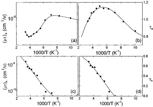
FIG. 1. The measured temperature dependence of the mobility-lifetime product and the light-intensity exponent of the electrons [(a) and (b)] and holes [(c) and (d)] in our *a*-Si:H samples. The curves are guides to the eye.
