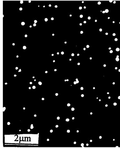
FIG. 1. SEM image of diamond nucleation for 35 min without bias.
