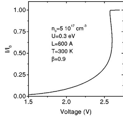
FIG. 6. S-type current-voltage characteristics for the barrier structure in Fig. 1.
