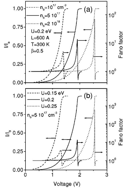
FIG. 3. Current-voltage characteristics and Fano factors for the barrier structure in Fig. 1 for different  $n_b$  (a) and different  $U$  (b).
