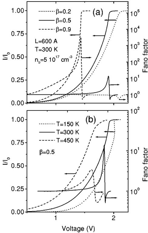
FIG. 4. Current-voltage characteristics and Fano factors for the barrier structure in Fig. 1 for different  $\beta$  (a) and for different  $T$  (b).
