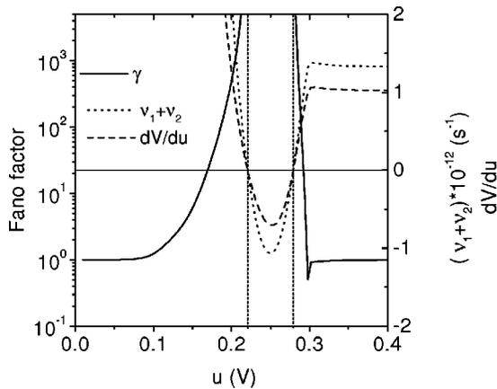
FIG. 8. Fano factor  $\gamma$ , inverse lifetime ( $\nu_1 + \nu_2$ ), and differential voltage drop  $dV/du$  as a function of the voltage drop between the emitter and the barrier  $u$  for the barrier structure in Fig. 1 in the presence of S-type current instability. The structure parameters are the same of those in Fig. 6.
