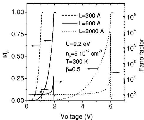
FIG. 5. Current-voltage characteristics and Fano factors for the barrier structure in Fig. 1 for different  $L$ .
