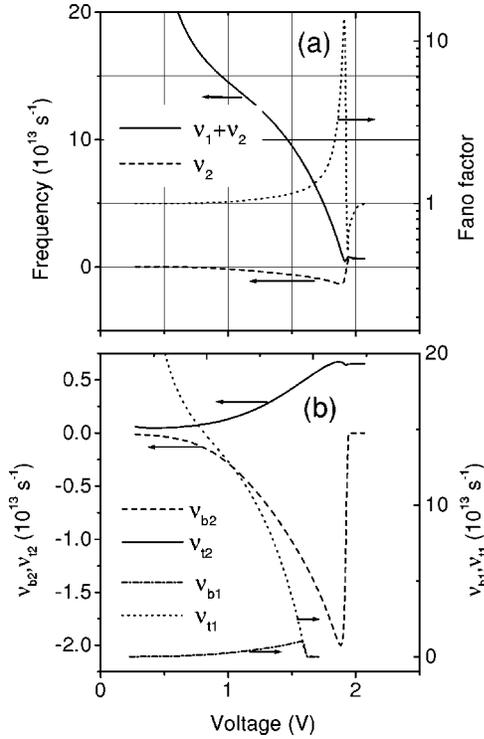
FIG. 7. Inverse lifetimes ( $\nu_1 + \nu_2$ ),  $\nu_2$  (a), and relevant rates  $\nu_{bi}$ ,  $\nu_{ii}$  ( $i=1,2$ ) (b) for the barrier structure in Fig. 1 with  $n_b=5 \times 10^{17}$  cm<sup>-3</sup>,  $U=0.2$  eV,  $L=600$  Å,  $T=300$  K, and  $\beta=0.5$ .
