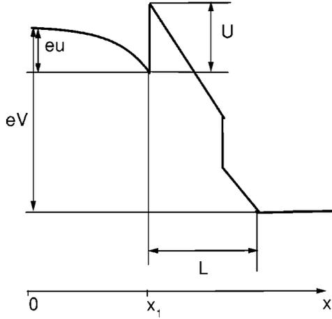
FIG. 1. Sketch of the band diagram of the single barrier structure considered here. Contact resistance at the terminals is neglected for simplicity.
