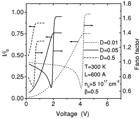
FIG. 9. Current-voltage characteristics and Fano factors for the single barrier structure in Fig. 1 with a constant barrier transparency for different values of the transmission coefficient  $D$ .
