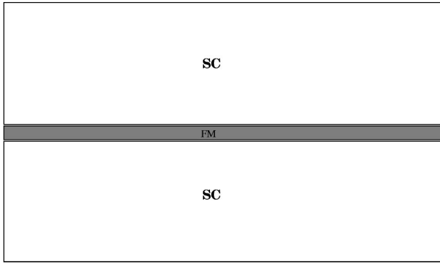
FIG. 1. Thin ferromagnetic film between bulk superconductors (schematic).
