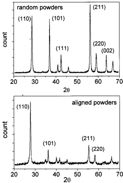
FIG. 2. X-ray-diffraction patterns of the random and aligned powders.
