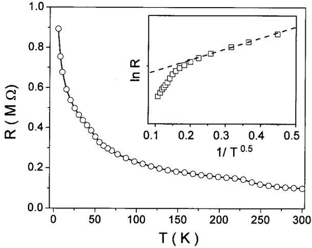
FIG. 5. Temperature dependence of the resistance  $R$ . Inset plots  $\ln R$  as a function of  $1/T^{1/2}$ .
