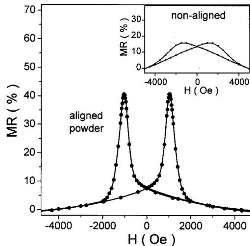
FIG. 4. TMR of the aligned powders at  $T = 5$  K. Inset shows the MR at 5 K of cold-pressed powders with random orientation, over the same field range.
