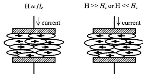
FIG. 1. Aligned magnetic moments of  $\text{CrO}_2$  powders and the structure of transport measurement.
