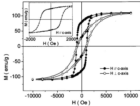
FIG. 3. The hysteresis loops of the aligned powders at  $T = 5$  K: field parallel to the easy axis ( $\bullet$ ) and perpendicular to the easy axis ( $\circ$ ). Inset shows the hysteresis loop (field applied parallel to the easy axis) over the smaller field range.
