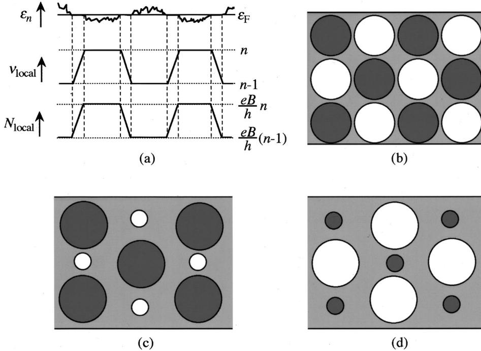
FIG. 5. (a) Schematic representation of the Landau-level energy, the local filling factor, and the local electron density. (b)–(d) Schematic representation of electron systems in high magnetic fields. It breaks up into incompressible regions in  $\nu=n$  IQH state (dark shaded) and incompressible regions in  $\nu=n-1$  IQH state (white), which are surrounded by compressible regions (light shaded). (b) Near the level center of Landau level. (c) Above the level center. (d) Below the level center.
