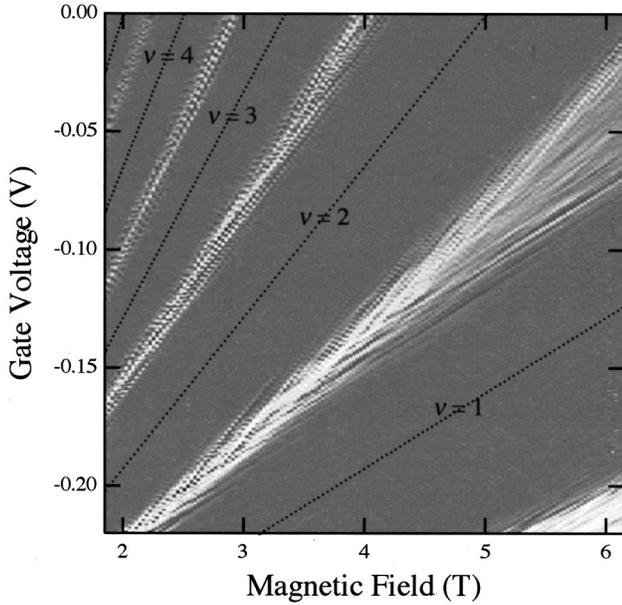
FIG. 3. Gray-scale plot of differential resistance in sweep of  $V_G$  and  $B$ . Lighter color represents larger value. The dark dotted lines represent integer filling of Landau level.
