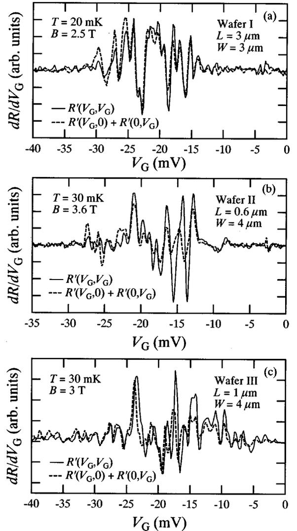
FIG. 2. IQH transition for the total system in differential resistance  $R'(V_G, V_G)$ , obtained by biasing both of the gates GL and GR simultaneously (solid line). The numerical sum of the single-gate spectrum for GL and that for GR (dashed line). (a)  $L = W = 3 \mu\text{m}$ , wafer I. (b)  $L = 0.6 \mu\text{m}$ ,  $W = 4 \mu\text{m}$ , wafer II. (c)  $L = 1 \mu\text{m}$ ,  $W = 4 \mu\text{m}$ , wafer III.
