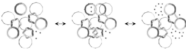
FIG. 11. From left to right: when the cut is translated in \mathbf{E}_\perp glue atoms become part of B or M(M') clusters; the clusters rearrange in space through a relatively few number of atom jumps. Observe, on the right, how some glue atoms are arranged in clusters that preclude the formation of either B or M(M') clusters.
