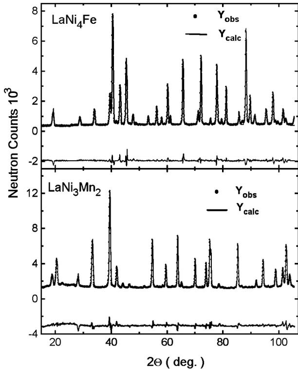
FIG. 2. The typical neutron diffraction patterns of  $\text{LaNi}_4\text{Fe}$  at 20 K and  $\text{LaNi}_3\text{Mn}_2$  at 30 K. The bottom curves are the difference between experimental data and refinement data.
