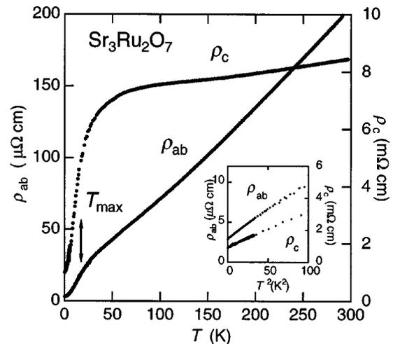
FIG. 3. The electrical resistivity of FZ crystals of  $\text{Sr}_3\text{Ru}_2\text{O}_7$  above 0.3 K. Both  $\rho_{ab}$  and  $\rho_c$  are shown. The inset shows the low-temperature electrical resistivity against the square of temperature  $T^2$ .
