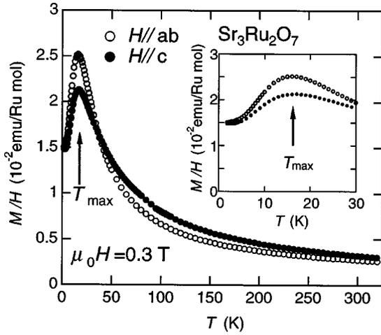
FIG. 1. The magnetic susceptibility of FZ crystals of  $\text{Sr}_3\text{Ru}_2\text{O}_7$  under 0.3 T field above 2 K. The inset shows the low-temperature magnetic susceptibility against temperature  $T$ .
