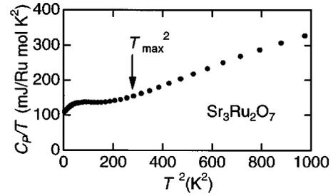
FIG. 2. The specific heat divided by temperature  $C_p/T$  of FZ crystals of  $\text{Sr}_3\text{Ru}_2\text{O}_7$  above 2 K.  $C_p/T$  is plotted against  $T^2$ .
