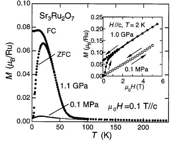
FIG. 4. The pressure dependence of magnetization  $M(T)$  for  $H \parallel c$ . Obvious ferromagnetic ordering appears at about 70 K under 1 GPa pressure. The inset shows the field dependence of magnetization  $M(H)$  under 0.1 MPa and 1 GPa pressures.
