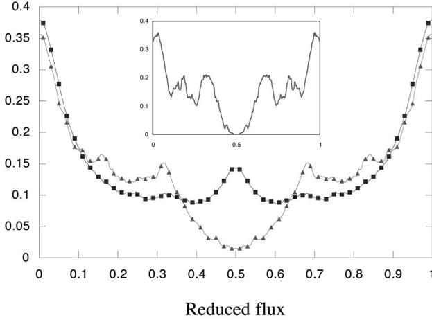
FIG. 2. Averaged transmission coefficient  $\langle T(k,f) \rangle_k / N_{in}$  as a function of the reduced flux for a  $(8 \times 8)$  square lattice (square) and a piece of the  $\mathcal{T}_3$  network (triangle) with 75 sites. Input and output channels are connected as displayed in Fig. 1. Inset: Averaged transmission coefficient for the  $\mathcal{T}_3$  network with one input channel at the center of the network.
