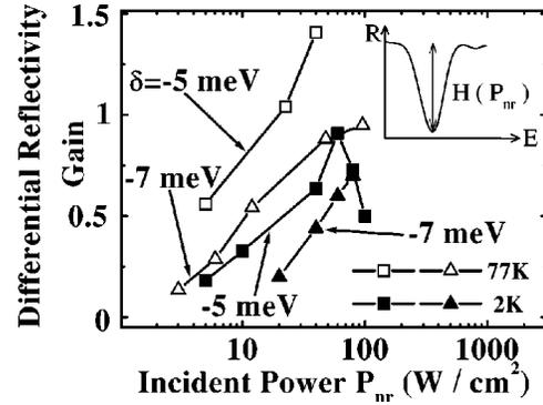
FIG. 4. Differential reflectivity gain (as defined in the text) as a function of  $P_{nr}$  for two temperatures and detunings.
