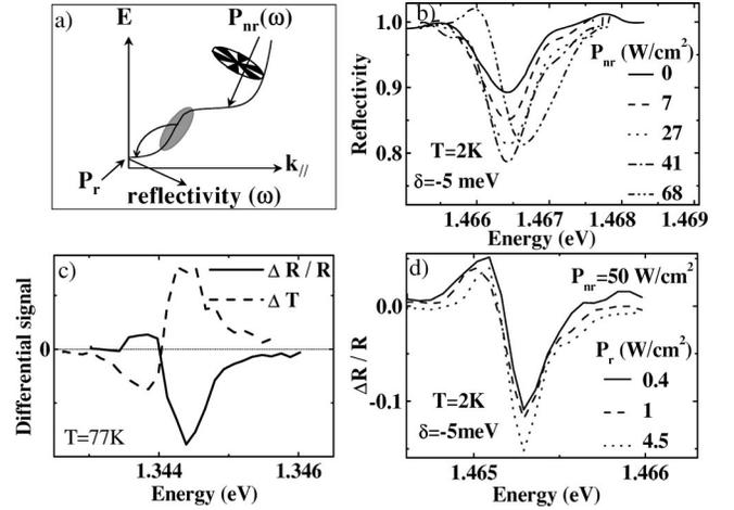
FIG. 2. (a) Schematic setup for differential reflectivity measurements. (b) Reflectivity spectra for various  $P_{nr}$ ,  $P_r = 0.2 \text{ W/cm}^2$ . (c) Simultaneous measurement of the relative reflectivity change and differential transmission. (d) Relative reflectivity change for  $P_{nr} = 50 \text{ W/cm}^2$  and various  $P_r$ .
