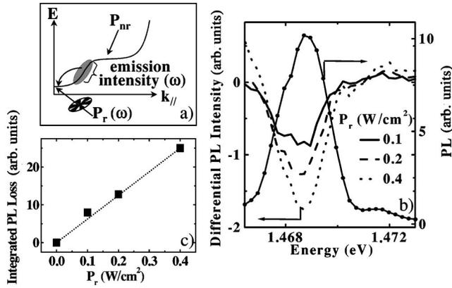
FIG. 3. (a) Schematic setup for differential PL measurements. (b) Right axis: PL spectrum measured between  $\theta=10^\circ$  and  $20^\circ$  with  $P_{nr}=8$  W/cm $^2$  and  $P_r=0$ . Left axis: Differential PL spectra between  $\theta=10^\circ$  and  $20^\circ$  for  $P_{nr}=8$  W/cm $^2$  and various  $P_r$ . The same units are used for right and left axis. (c) Integrated PL loss as a function of  $P_r$ . The dotted line is a linear fit.  $\delta=-5$  meV and  $T=2$  K.
