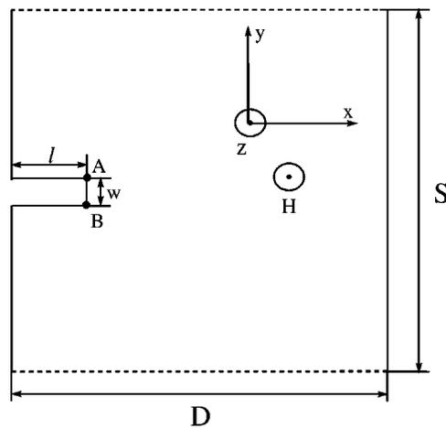
FIG. 1. The bulk superconductor ( $-\infty < y < \infty, -\infty < z < \infty$ ) with surface defect (chain of defects—see text) in an external magnetic field  $\mathbf{H} = (0, 0, H)$ .
