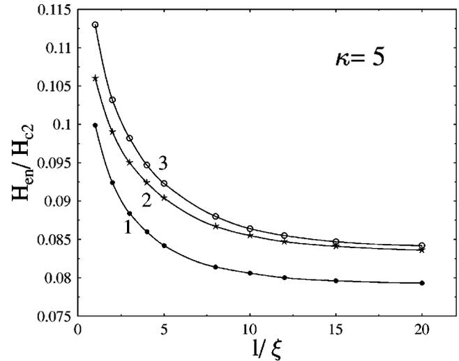
FIG. 3. Dependence of field  $H_{\text{en}}$  on a defect length at  $w = \text{const}$  for type-II bulk superconductor ( $\kappa=5$ ), obtained from the results of numerical calculation of Eqs. (1) and (2). Curve 1 (dots) is for a defect with  $w=1\xi$ , curve 2 (stars) is for  $w=2\xi$ , and curve 3 (circles) is for  $w=3\xi$ .
