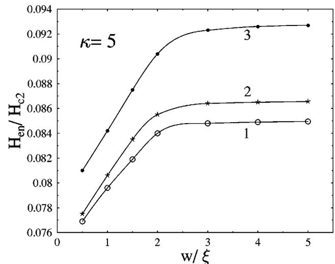
FIG. 4. Dependence of field  $H_{\text{en}}$  on a defect width at  $l = \text{const}$  for a type-II bulk superconductor ( $\kappa=5$ ), obtained from the results of numerical calculation of Eqs. (1) and (2). Curve 1 (circles) is for a defect with  $l=15\xi$ , curve 2 (stars) is for  $l=10\xi$ , and curve 3 (dots) is for  $l=5\xi$ .
