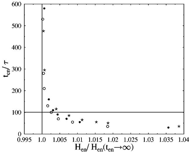
FIG. 2. Vortex entry time  $t_{\text{en}}$  as a function of an applied magnetic field  $H$ . Circles are for  $\kappa=7$ , dots for  $\kappa=5$ , and stars for  $\kappa=2$ . The results were obtained for a defect with size:  $l=2\lambda$ ;  $w=\xi$ .
