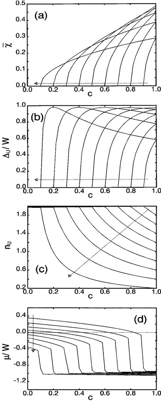
FIG. 7. The order parameter  $\bar{\chi}$  (a), the local pairing potential on  $U$  site  $\Delta_U$  (b), and the local charge on  $U$  site  $n_U$  (c) and the chemical potential  $\mu$  (d) plotted versus concentration  $c$  for  $U/W = -2.0$  and several values of  $n$  ( $n = 1.8, 1.6, 1.4, 1.2, 1.0, 0.8, 0.6, 0.4, 0.2$  — the direction of  $n$  changing is pointed out by the arrow).
