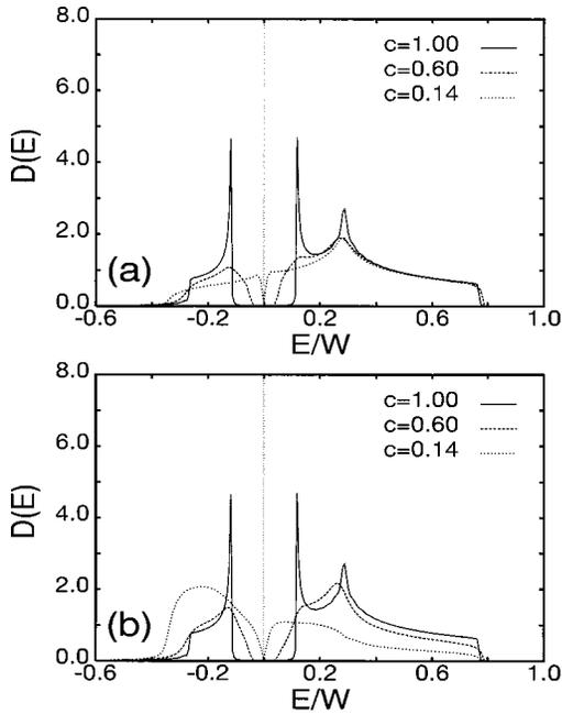
FIG. 9. The averaged quasiparticle densities of states (a) and the local densities of states on  $U$  site (b) for  $U/W = -0.5$ ,  $n = 0.4$  and several values of  $c$  specified in the figures.
