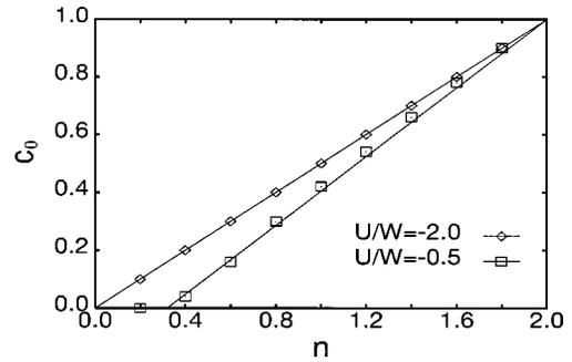
FIG. 10. The critical concentration of negative centers  $c$  versus band filling  $n$  for  $U/W = -2.0$  and  $-0.5$ .
