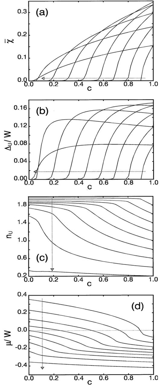
FIG. 8. The order parameter  $\bar{\chi}$  (a), the local pairing potential on  $U$  site  $\Delta_U$  (b), and the local charge on  $U$  site  $n_U$  (c) and the chemical potential  $\mu$  (d) plotted versus concentration  $c$  for  $U/W = -0.5$  and several values of  $n$  ( $n = 1.8, 1.6, 1.4, 1.2, 1.0, 0.8, 0.6, 0.4, 0.2$  — the direction of  $n$  changing is pointed out by the arrow).
