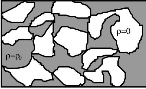
FIG. 1. A mixture of normal, with resistance  $\rho = \rho_0$ , and super, with  $\rho = 0$ , conductors.
