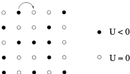
FIG. 2. The propagation of Cooper pairs between negative  $U < 0$  centers by hopping from site to site, where  $U = 0$  on the intermediate sites.
