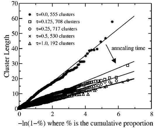
FIG. 2. Exponential plot of cluster length distributions at various times during simulated evolution of the grain structure in a thin film strip with  $w/D_{50}=1.0$ . Solid lines represent the best-fitting exponential distributions. The plot is consistent with the structure reaching a steady state where the average cluster length is constant.
