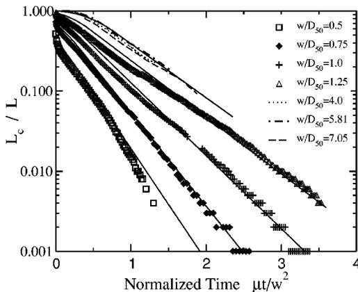
FIG. 5. Evolution of the normalized total cluster length  $L_c = L_c/L$  with  $\tau = \mu t/w^2$ . The plots coincide for initially polygranular lines ( $w/D_{50} > 2$ ). Solid lines represent the evolution predicted using the analytic model.
