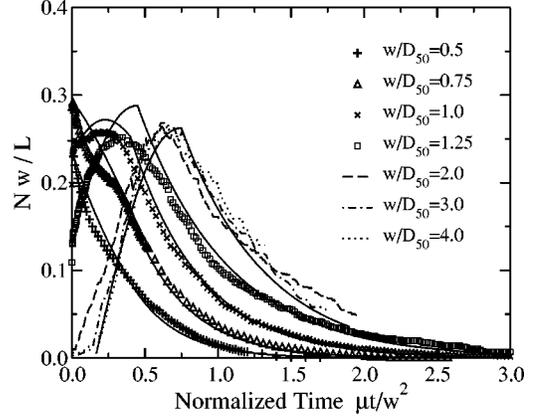
FIG. 6. Simulated evolution of the normalized number of clusters  $N = Nw/L$  with  $\tau = \mu t/w^2$ . The plots overlap for initially polygranular lines. Solid lines represent the predictions of the analytic model.
