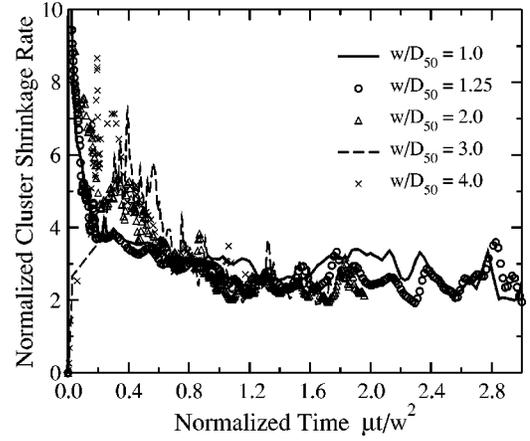
FIG. 3. Evolution of the normalized cluster shrinkage rate  $\underline{v} = -(1/N)dL_c/d\tau$  with  $\tau = \mu t/w^2$ . The plots coincide for initially polygranular lines ( $w/D_{50} > 2$ ), confirming that the shrinkage rate is proportional to  $\mu/w$ .
