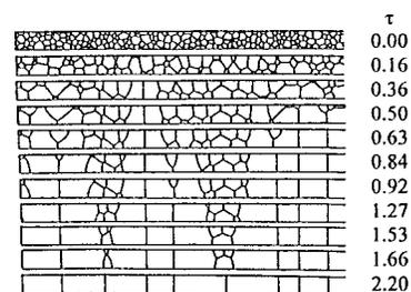
FIG. 1. Evolution of the grain structure within a strip with  $w/D_{50} = 3.0$ .  $w$  is the linewidth and  $D_{50}$  is the median grain size in the film from which the line is etched.  $\tau = \mu t/w^2$  is the normalized dimensionless time.
