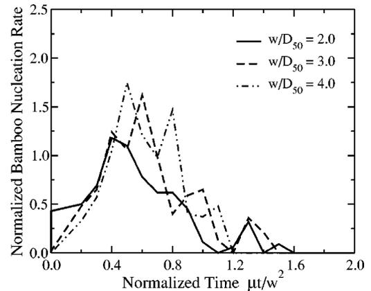
FIG. 4. Evolution of the normalized bamboo nucleation rate  $(1/L_c)dN_b/d\tau$  with  $\tau = \mu t/w^2$ . These plots have been obtained after averaging highly variable instantaneous rates over longer times. The plots coincide within statistical variations for initially polygranular lines ( $w/D_{50} > 2$ ) showing that bamboo nucleation is only significant during the nucleation phase and that the nucleation rate is proportional to  $\mu/w^3$ .
