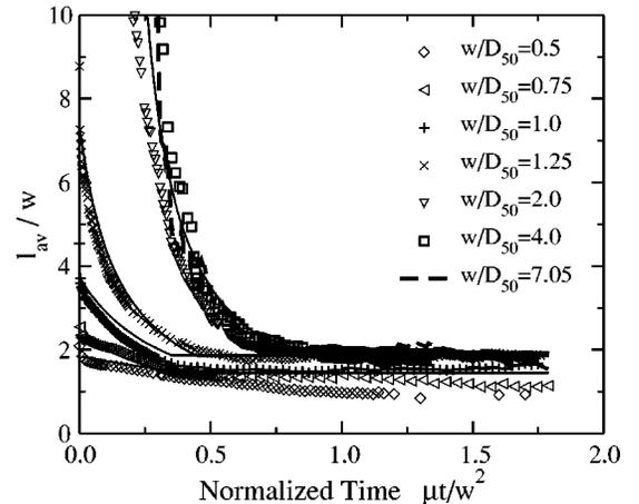
FIG. 7. Simulated evolution of the normalized average cluster length  $l_{av} = l_{av}/w$  with  $\tau = \mu t/w^2$ . Solid lines represent the predictions of the analytic model.
