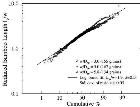
FIG. 8. Log-normal plot of normalized bamboo grain length  $l_b/w$  distributions in the bamboo structures, resulting from simulated prolonged annealing of polygranular strips with different widths. The overlapping curves for different values of  $w/D_{50}$  show that the distribution of the values of  $l_b/w$  is linewidth-independent. The solid line represents the best-fitting log-normal distribution.
