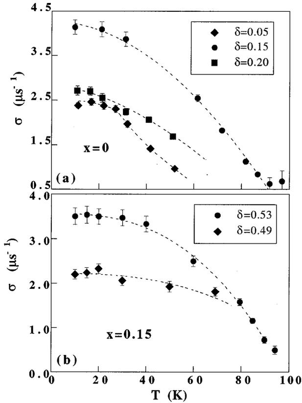
FIG. 2. Temperature dependence of the muon relaxation rate  $\sigma$ , for Hg-1201 ceramics with different doping level, for  $x=0$  (a) and  $x=0.15$  (b).
