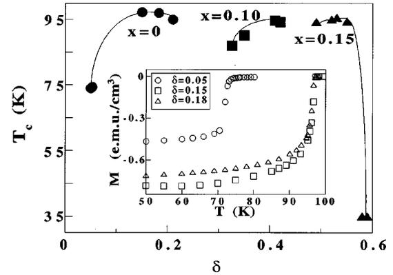
FIG. 1. Evolution of the critical temperature with oxygen excess  $\delta$ , for samples with different Re content  $x$ . (Inset) Low field diamagnetic transitions of  $x=0$  samples with different oxygen doping.
