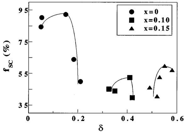
FIG. 4. Dependence of the superconducting volume fraction  $f_{SC}$  on the oxygen excess  $\delta$ , for samples with  $x=0, 0.10$ , and  $0.15$ .
