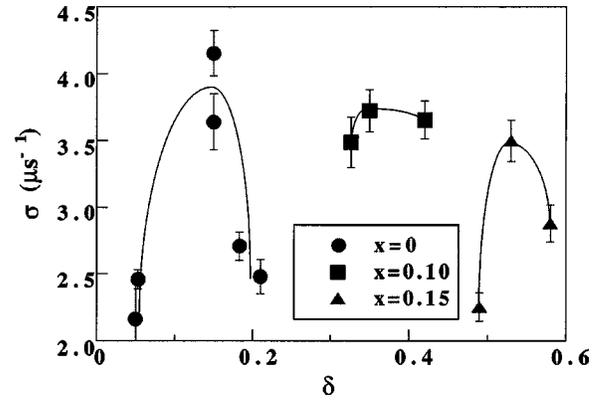
FIG. 3. Values of the low temperature ( $T=10$  K) muon relaxation rate  $\sigma$  for superconducting Hg-1201 samples with different Re and oxygen contents.
