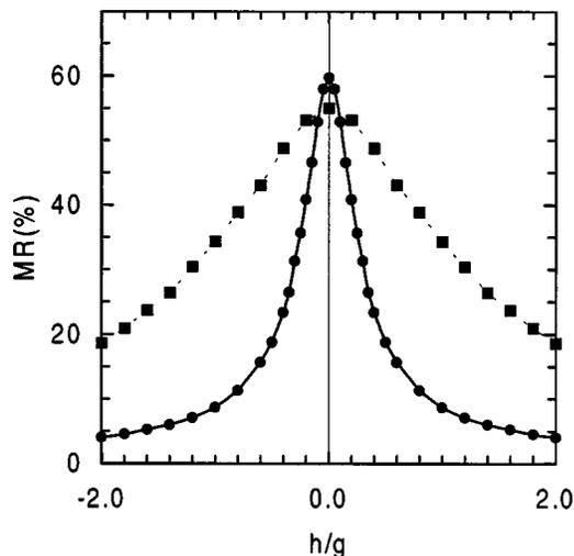
FIG. 5. Field dependence of anhysteretic magnetoresistance for a dipolar sample (squares) and for a noninteracting sample (circles). Parameters:  $p=30\%$  ( $\text{Co}_{16}\text{Cu}_{84}$ ) and  $T=82$  K. Monodisperse samples.
