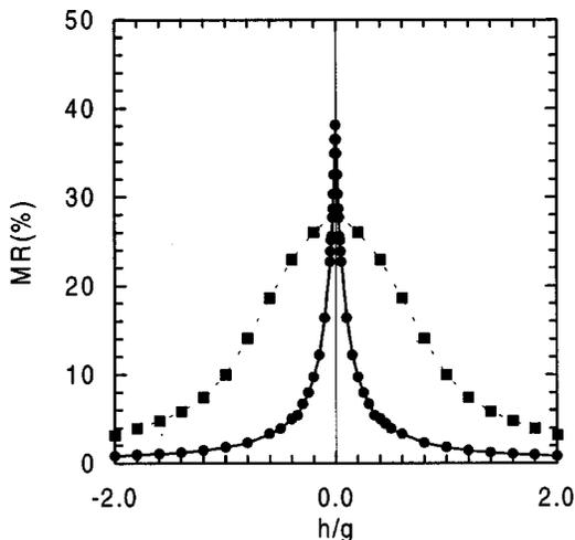
FIG. 12. Field dependence of anhyseretic magnetoresistance of a dipolar sample (squares) and a noninteracting sample (circles). Parameters:  $p=30\%$  ( $\text{Co}_{16}\text{Cu}_{84}$ ) and  $T=82$  K. Coalescence is allowed in both samples.
