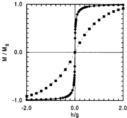
FIG. 11. Anhyseretic magnetization curve for a dipolar system (squares) and magnetization curve for a noninteracting system (circles). Parameters  $p=30\%$  ( $\text{Co}_{16}\text{Cu}_{84}$ ) and  $T=82$  K. Coalescence is allowed in both systems.
