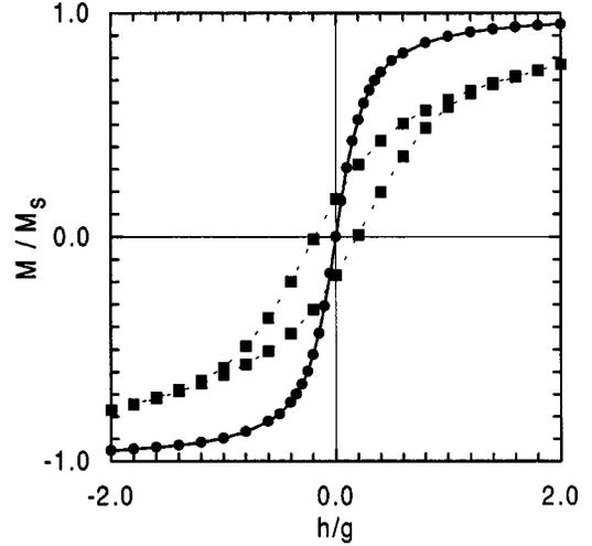
FIG. 2. Hysteresis loop for a dipolar system (squares) and magnetization curve for a noninteracting system (circles). Parameters  $p = 30\%$  ( $\text{Co}_{16}\text{Cu}_{84}$ ) and  $T = 82 \text{ K}$ . Monodisperse samples.
