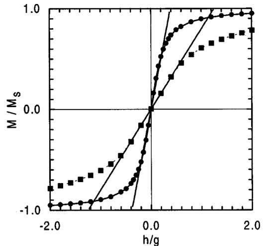
FIG. 3. Anhysteretic magnetization curve for a dipolar system (squares) and magnetization curve for a noninteracting system (circles). Straight line fits to the low-field data are shown. Parameters  $p = 30\%$  ( $\text{Co}_{16}\text{Cu}_{84}$ ) and  $T = 82 \text{ K}$ . Monodisperse samples.
