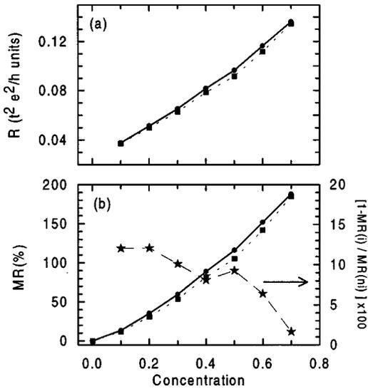
FIG. 7. Concentration dependence of (a) the zero-field resistance and (b) the zero-field magnetoresistance of dipolar (squares) and noninteracting (circles) monodisperse  $\text{Co}_x\text{Cu}_{1-x}$  samples. The percentage change of the MR due to dipolar interactions is also shown (stars) and  $\text{MR}(\text{ni})$ ,  $\text{MR}(\text{i})$  denote the MR values for the noninteracting and interacting systems, respectively. Parameters:  $T=8$  K.
