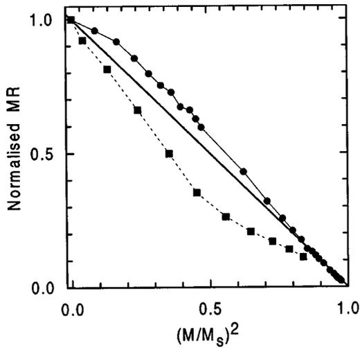
FIG. 14. Normalized anhysteretic magnetoresistance versus reduced magnetization for a dipolar sample (squares) and for a non-interacting sample (circles). Parameters:  $p=30\%$  ( $\text{Co}_{16}\text{Cu}_{84}$ ) and  $T=82\text{ K}$ . Coalescence is allowed in both samples.
