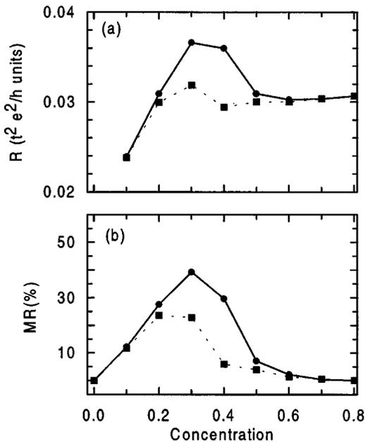
FIG. 10. Concentration dependence of (a) the zero-field resistance and (b) the zero-field magnetoresistance of dipolar (squares) and noninteracting (circles)  $\text{Co}_x\text{Cu}_{1-x}$  samples. Coalescence is allowed in all samples. Parameters:  $T = 82$  K.
