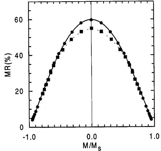
FIG. 6. Anhysteretic magnetoresistance versus reduced sample magnetization for a dipolar sample (squares) and for a noninteracting sample (circles). Parameters:  $p=30\%$  ( $\text{Co}_{16}\text{Cu}_{84}$ ) and  $T=82$  K. Monodisperse samples.
