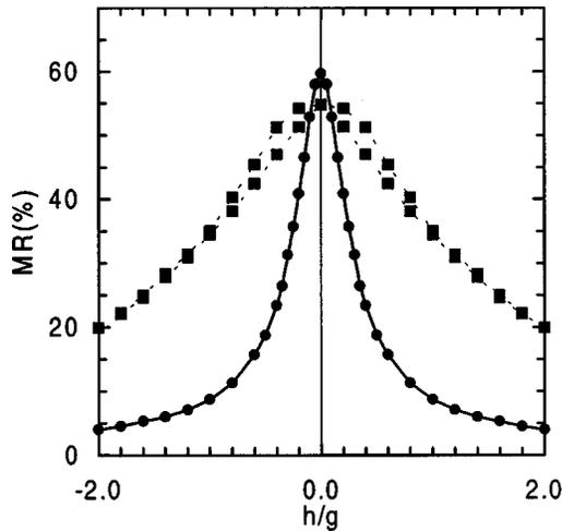
FIG. 4. Field dependence of hysteretic magnetoresistance for a dipolar sample (squares) and for a noninteracting sample (circles). Parameters:  $p=30\%$  ( $\text{Co}_{16}\text{Cu}_{84}$ ) and  $T=82$  K. Monodisperse samples.
