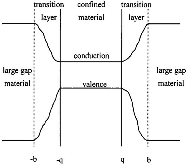
FIG. 2. General band scheme of the quantum well embedded in an oxide.
