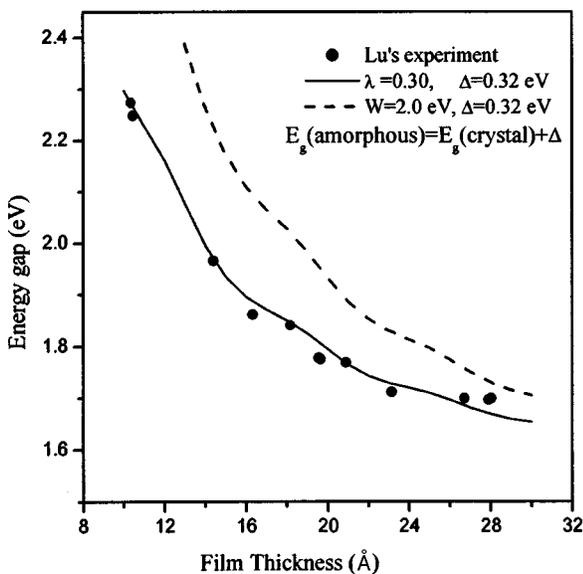
FIG. 3. Dependence of the energy gap on the well thickness for the amorphous silicon quantum well.
