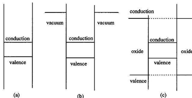
FIG. 1. Band diagrams for (a) an infinite energy barrier, (b) a free-standing film surrounded by vacuum, and (c) a quantum well embedded in a large-energy-gap material.
