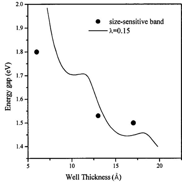
FIG. 4. Dependence of the energy gap on the well thickness for the silicon quantum well fabricated from a SIMOX wafer.
