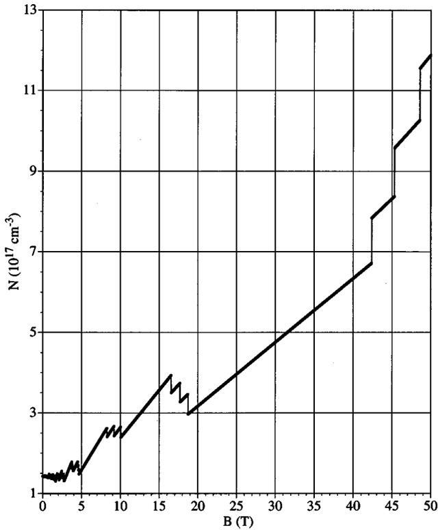
FIG. 4. Carrier density versus magnetic field;  $T=0$ , film thickness is 915 Å.
