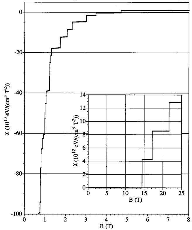
FIG. 8. Magnetic susceptibility versus magnetic field;  $T=0$ , film thickness is 525 Å; inset 410 Å.
