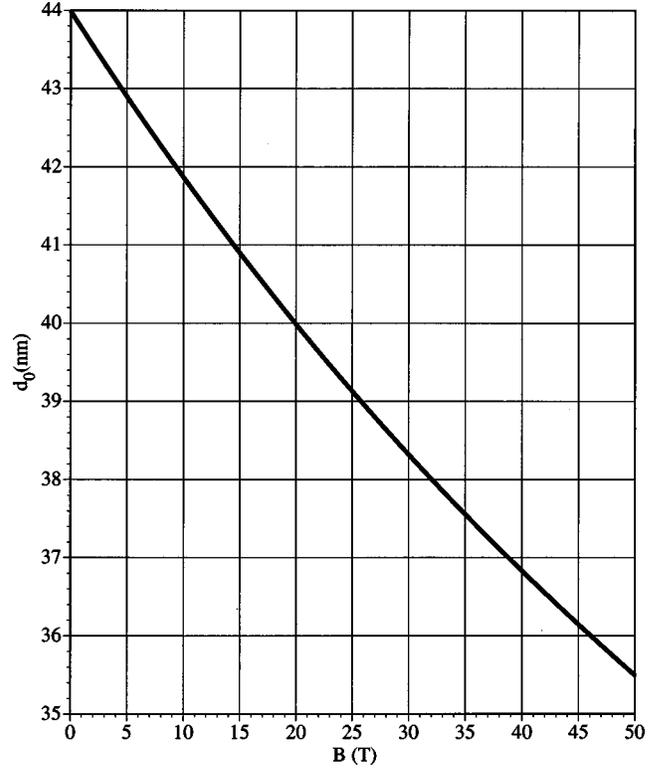
FIG. 1. Semiconductor-semimetal transition diagram: film thickness  $d_0$  (where semiconductor-semimetal transition occurs) versus magnetic field.
