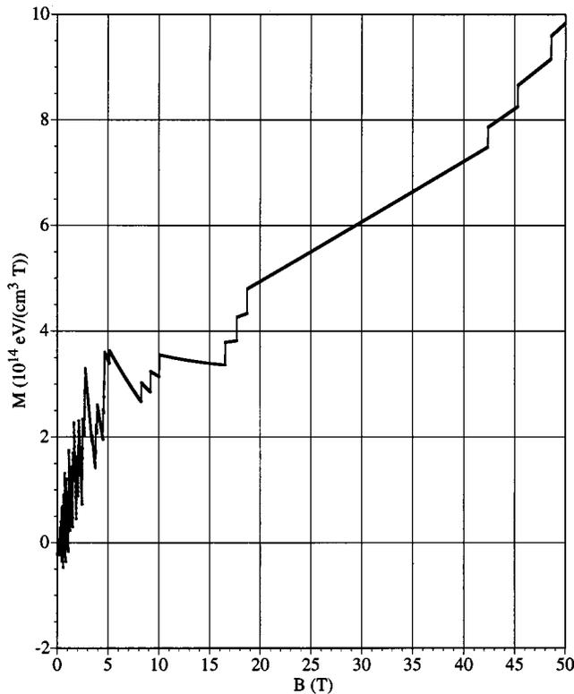
FIG. 7. Magnetization versus magnetic field;  $T=0$ , film thickness is 915 Å.
