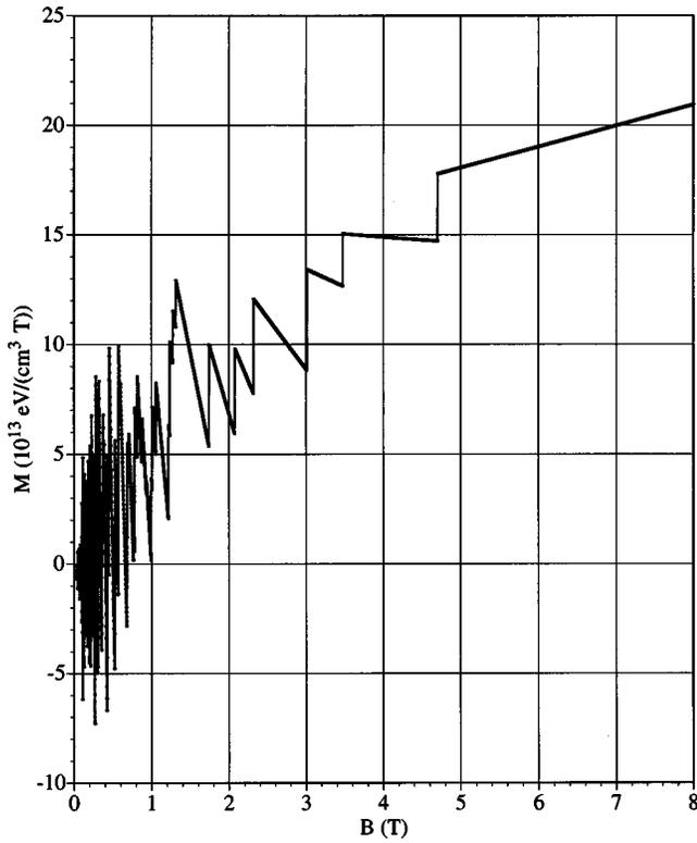
FIG. 6. Magnetization versus magnetic field;  $T=0$ , film thickness is 525 Å.
