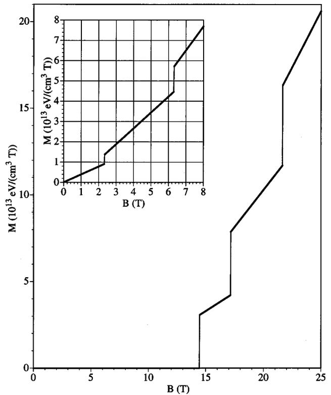
FIG. 5. Magnetization versus magnetic field;  $T=0$ , film thickness is 410 Å; inset 440 Å.
