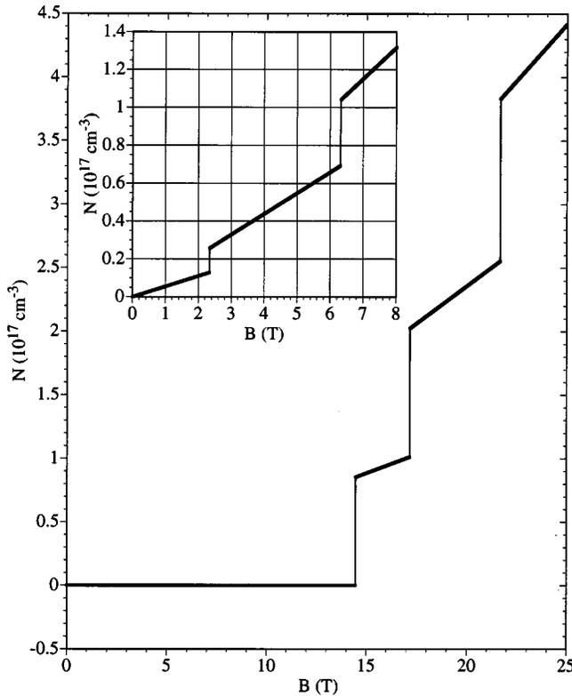
FIG. 2. Carrier density versus magnetic field;  $T=0$ , film thickness is 410 Å; inset 440 Å.
