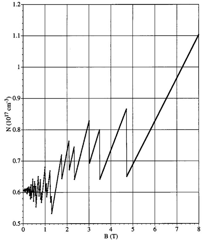
FIG. 3. Carrier density versus magnetic field;  $T=0$ , film thickness is 525 Å.
