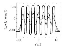
FIG. 7. The equilibrium current  $I_{eq}$  plus the regular current  $I_r$  vs voltage.  $L=10\xi_o$ ,  $\phi=\pi/2$ , D=0.8,  $\epsilon=0.05$ . Solid line: T=0, dashed dotted:  $kT=0.04\Delta$ , dashed:  $kT=0.07\Delta$ . The regular current jumps alternating by  $\pm \delta I_r$  every time the voltage is equal to the energy of an Andreev resonance. For  $kT \gg \hbar v_F/L$  and  $eV > \Delta$  the current  $I_{eq}+I_r=I_{eq}^c$ .
