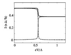
FIG. 5. The currents  $I_{eq}+I_r$  (dash dotted),  $I_a$  (dashed), and the total Josephson current  $I_{eq}+I_r+I_a$  (solid) in the horizontal leads 2 and 3 as a function of voltage V at T=0 for a short junction L = 0 with D=0.8,  $\phi=3\pi/4$ ,  $\epsilon=0.01$ , and  $\sigma=-1$ . The total current is  $I_{eq}$  for  $eV < E_0^-$  and  $\delta I_a$  for  $eV > E_0^-$ .
