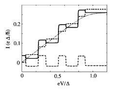
FIG. 9. The total current  $I = I_{eq} + I_r + I_a$  as a function of voltage. At zero temperature we have  $I_r + I_{eq}$  (dash dotted),  $I_a$  (dashed), and the total current  $I_r + I_{eq} + I_a$  (solid). The total current for temperatures  $kT \gg \hbar v_F/L$  is plotted (dotted). Junction parameters are D = 0.8,  $\phi = 3 \pi/4$ ,  $L = 20\xi_0$ ,  $\epsilon = 0.01$ , and  $\sigma = -1$ .
