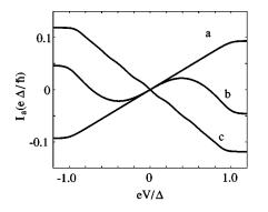
FIG. 10. The asymmetric anomalous current  $I_a$  vs voltage for different asymmetries (a)  $l=0\xi_0$ , (b)  $l=2\xi_0$ , and (c)  $l=40\xi_0$  for  $kT \gg \hbar v_F/L$ , D=0.8,  $\epsilon=0.05$ ,  $L=60\xi_0$ ,  $\phi=\pi/4$ , and  $\sigma=-1$ . The IVC is changed dramatically already for as small asymmetry  $l \sim \xi_0$ , if the phase difference  $-\pi/2 < \phi < \pi/2$ .
