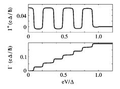
FIG. 2. The current voltage characteristics (IVC) for  $I^+$  (upper) and  $I^-$  (lower) for a junction with seven Andreev levels for  $0 < E < \Delta$ . The currents jump every time the voltage eV is equal to the energy of an Andreev level, typical for resonant transport.
