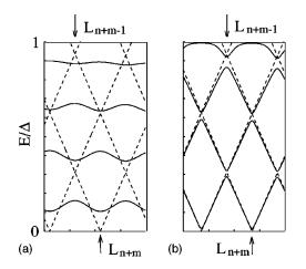
FIG. 12. The Andreev levels (solid) and the normal electron and hole resonances (dotted) as a function of length *L* of the junction with four Andreev levels in (a) weak resonance limit  $R_b \ll 1$  (b) strong resonance limit  $R_b \sim 1$ . The lengths of two subsequent intersections of normal resonances  $L_{n+m}$  and  $L_{n+m-1}$  are shown with arrows.
