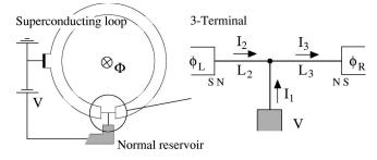
FIG. 1. A schematic picture of the three-terminal SNS junction setup under consideration, with a normal reservoir attached to the normal part of the junction. The normal reservoir is connected to the superconducting loop (grounded) via a voltage source biased at V. The right figure shows a closeup of the junction area with the arrows showing the direction of the current flow in the junction.
