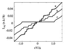
FIG. 14. The injection current in lead 1 as a function of voltage for (a)  $\phi = \pi/4$ , (b)  $\phi = 3\pi/4$ , and (c)  $\phi = \pi$ . Zero *T* (solid lines) and  $T = 0.05\Delta$  (dashed line) with D = 0.8,  $L = 10\xi_0$ , and  $\epsilon = 0.05$ . For  $eV > \Delta$  the slope of the IVC approaches the value of a normal junction.
