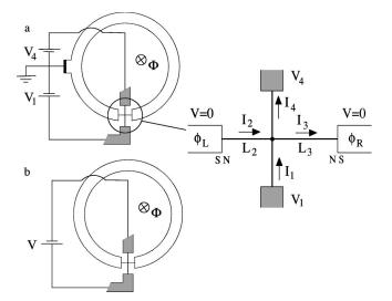
FIG. 18. Two different setups of the four terminal junction. In (a) the normal reservoirs are biased independently at  $V_1$  and  $V_4$  with respect to the superconducting loop (grounded), in (b) only the potential difference between the normal reservoirs, V, is determined. In the right figure, a close up of the junction area is shown, with the direction of the currents showed with arrows
