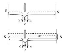
FIG. 17. The paths in the asymmetric junction giving the firstorder terms of the current. Electrons are drawn with solid lines, holes with dashed. The gray ellipse denotes the effective scatterer due to the three-lead connection. The upper paths give rise to a  $2\pi$ periodic component of the current, suppressed at finite temperature  $kT \gg \hbar v_F/L$ . The lower paths, time reversed, give rise to a  $\pi$  periodic component of the current, not suppressed by temperature.
