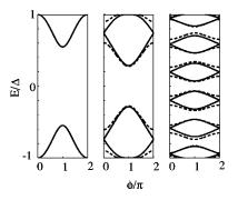
FIG. 4. Andreev bound state energies as a function of phase difference  $\phi$  for different lengths L=0 (left),  $L \sim \xi_0$  (middle), and  $L \gg \xi_0$  (right) of the junction with D=0.7. Solid lines are for a symmetric junction l=0, dashed for an asymmetric one. A gap opens up in the spectrum at  $\phi=0$  due to the asymmetry.
