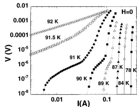
FIG. 1. The current-voltage curves as a function of temperature in ambient magnetic fields ( $<1$  Oe). The separate contribution of the GB (i.e., the foot of the transition) is apparent at intermediate temperatures.
