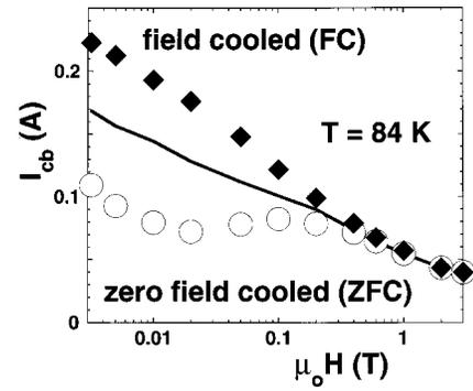
FIG. 4. From data such as Fig. 3, taken as a function of field, the  $I_{cb}$  for FC (solid symbols) and ZFC (open symbols) are shown. The solid line is the irreversible (i.e., permanent) change in  $I_{cb}$  found upon exceeding  $I_{cg}$  after ZFC.
