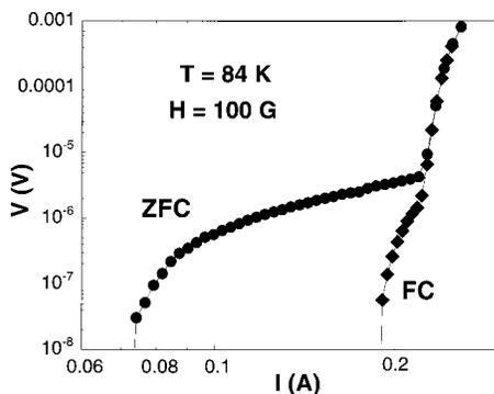
FIG. 3. The differences in  $I(V)$  between FC and ZFC for  $84 \text{ K}$  and  $100 \text{ Oe}$ .
