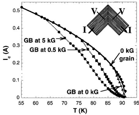
FIG. 2. The temperature dependences of  $I_{cb}$  for various applied fields that were perpendicular to the platelike shape (inset) and thus parallel to the GB plane and to the Cu-O planes of each arm. For the grains, the  $I_{cg}$  were virtually independent of field. Data were taken while cooling the sample in a field which was applied above the transition temperature,  $T_c$ .
