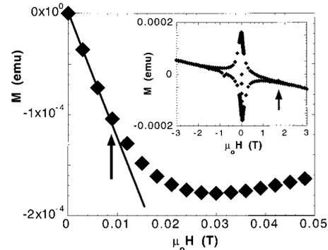
FIG. 5. The bulk magnetization of one half of a GB measured at  $77 \text{ K}$ . The deviation from the Meissner-like magnetization at  $\sim 0.01 \text{ T}$  (arrow) signals the entry of flux *into the grain* and the inset shows that the grains are reversible above about  $2 \text{ T}$  (arrow).
