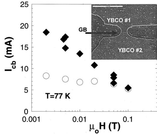
FIG. 6. Similar  $I_{cb}$  data as in Fig. 4, but here taken on a patterned GB on a coated conductor (inset), for FC (solid symbols) and ZFC (open symbols).
