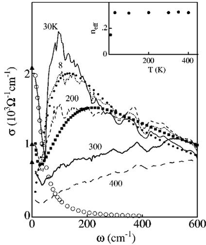
FIG. 3. Expansion in the FIR of the  $\sigma(\omega)$  of Fig. 2. The open circles are the best fit to a normal Drude term, given by Eq. (3), here proposed only for the 30 K curve. The dots and the squares are best fits of Eqs. (4) and (5) to data at 8 and 200 K, respectively. The triangles on the ordinate axis represent the values of  $\sigma_{dc}$  measured at the same temperatures, also reported in the inset of Fig. 1. The inset shows the spectral weight calculated from Eq. (2) (see text).
