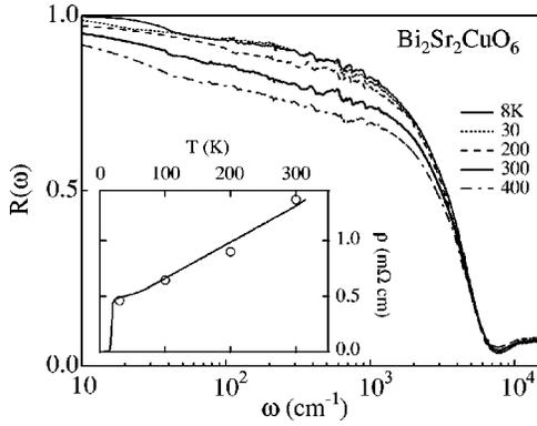
FIG. 1. Reflectivity  $R(\omega)$  of the BSCO film at five temperatures from 400 to 8 K. The inset shows the resistivity  $\rho(T)$  of the film from 300 to 4 K. The open circles are the  $\rho$  values obtained by extrapolating  $\sigma(\omega, T)$  in Fig. 3 to  $\omega=0$ .
