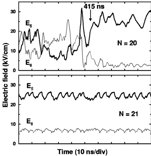
FIG. 2. Temporal variations of the electric fields in fifth and sixth barriers in the structures with 20 and 21 QW's.
