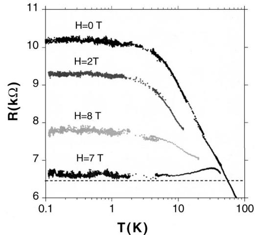
FIG. 3. The temperature dependence of the four-probe resistance for sample *S1* in the presence of a perpendicular magnetic field. The dotted line represents a resistance value of 6.45 k $\Omega$  ( $=h/4e^2$ ).
