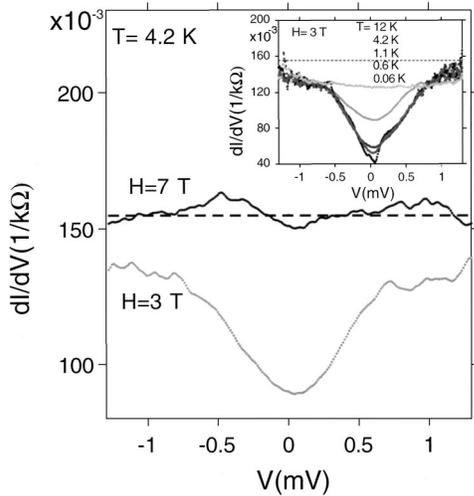
FIG. 4. The  $dI/dV$  curves for sample  $S1$  near the resistance maximum ( $H=7.0$  T) and minimum ( $H=3.0$  T) points at 4.2 K. Inset: the temperature dependence of the  $dI/dV$  curves at  $H=3.0$  T. The dotted line represents the resistance value of  $6.45$   $k\Omega$  ( $=h/4e^2$ ).
