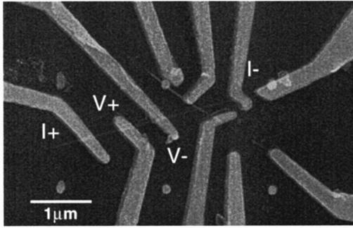
FIG. 1. Scanning electron microscope image of sample *S1* used in this study. The four electrodes used in the measurement are denoted in the figure.
