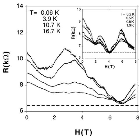
FIG. 2. The four-probe MR curves for sample *S1* in a perpendicular magnetic field with a bias current of 50 nA at various temperatures. Inset: the four-probe MR curves for sample *S2* in a perpendicular magnetic field with a bias current of 0.5 nA. The dotted line represents the resistance value of 6.45 k $\Omega$  ( $=h/4e^2$ ).
