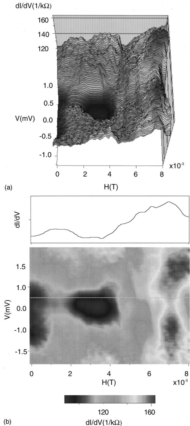
FIG. 5. (a) A perspective view of the  $dI/dV(V,H)$  curves for sample  $S1$  at 4.2 K as a function of bias voltage  $V$  and magnetic field  $H$ . (b) A top view of the  $dI/dV(V,H)$  curves for sample  $S1$  and the cross-sectional plot along the dotted line.
